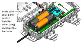
The mote contacts the network once the new batteries are installed. The green LED blinks quickly while the mote searches for a network to join and then blinks slowly while it completes the network registration. Once the mote has finished joining the network, the green LED turns off and the blue LED then blinks indefinitely while the mote is part of the network.
