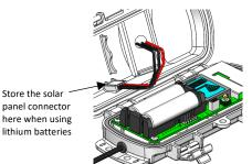
The mote contacts the network once the new batteries are installed. The green LED blinks quickly while the mote searches for a network to join and then blinks slowly while it completes the network registration. Once the mote has finished joining the network, the green LED turns off and the blue LED then blinks indefinitely while the mote is part of the network.
