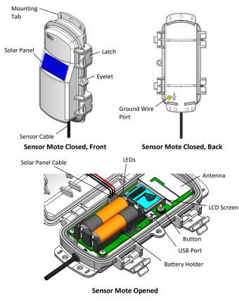
**Mounting Tab:** Use the tabs at the top and bottom of the mote to mount it (see *Deploying and Mounting*).
