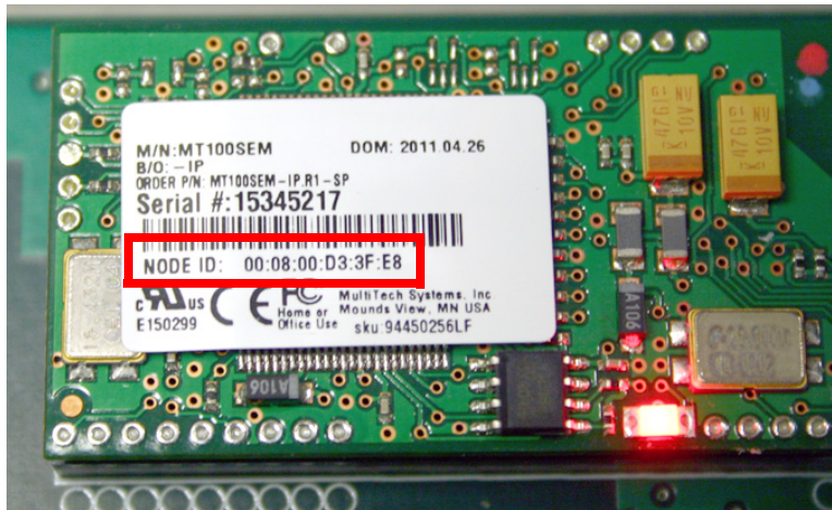
Figure 5-30 Locating the NODE ID (MAC address) on the ethernet modem
