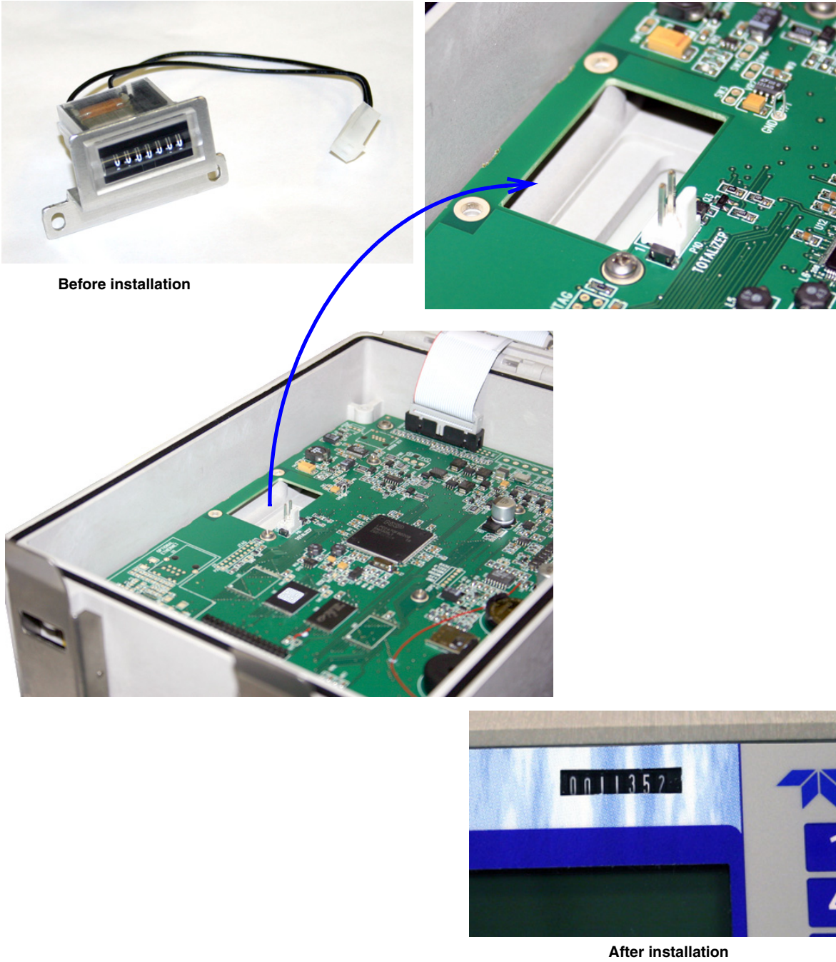
Figure 5-10 Optional non-resettable totalizer installation
