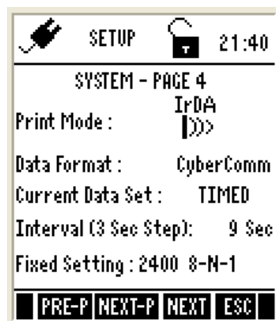
Figure 5: System Settings Page 4 – Wireless Serial Data Communication
