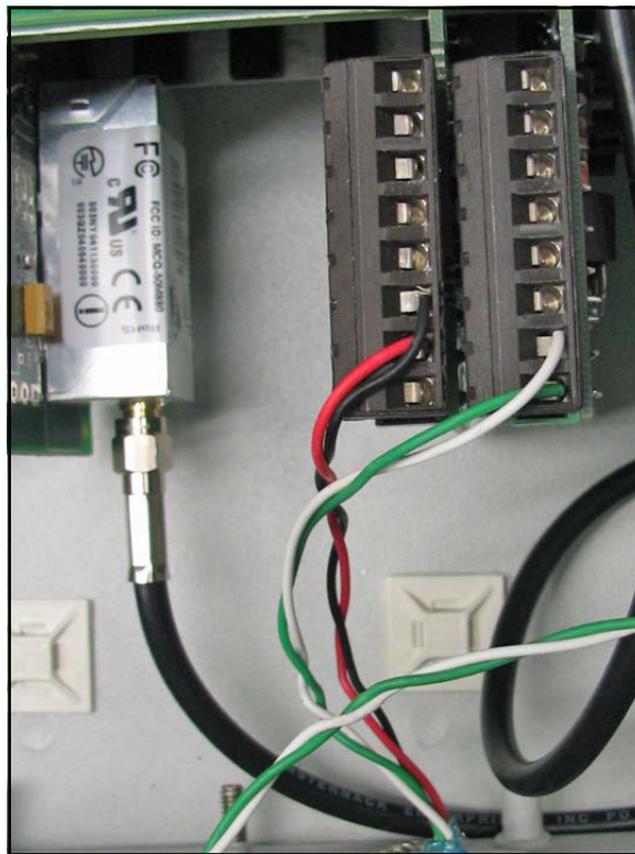
Figure 41: WI-FI Cable PC Board Connection
