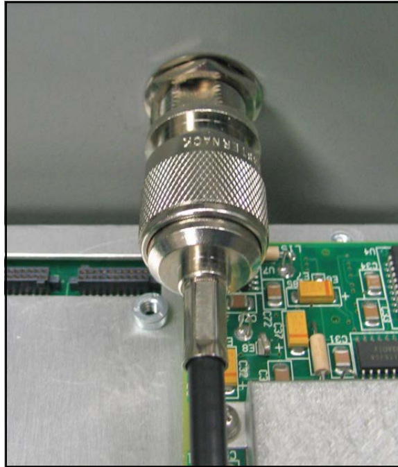
Figure 40: WI-FI Cable Antenna Connection
