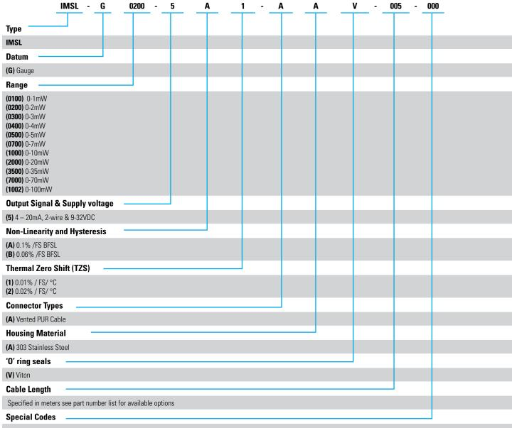
The IMSL pressure sensor was designed to be easily customized, and in addition to the standard options for electrical and mechanical configuration, the sensor can also be specially tailored to a particular OEM requirement and given a unique part number code.
