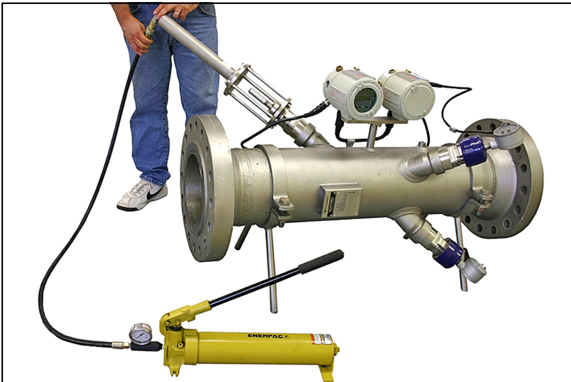
Figure 8: Connecting the Hydraulic Pump
