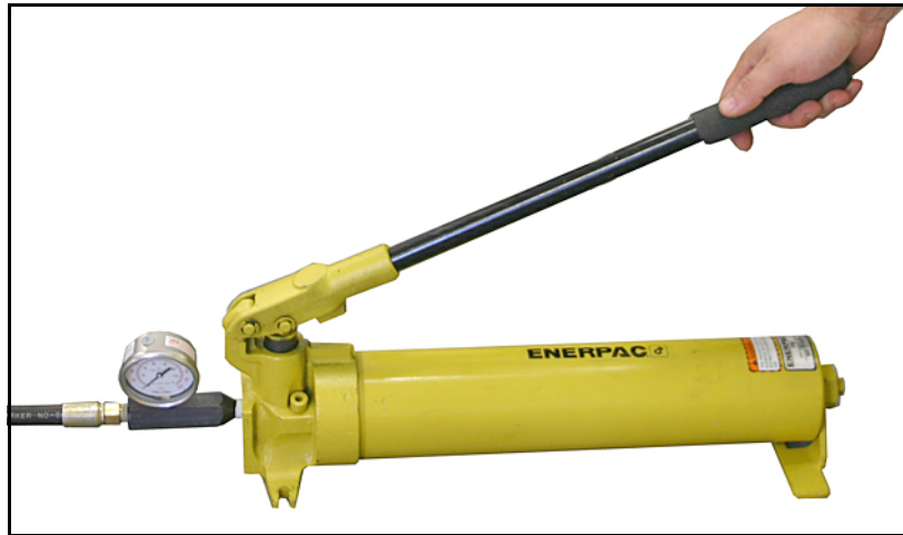
Figure 9: Pressurizing the Hydraulic Pump
