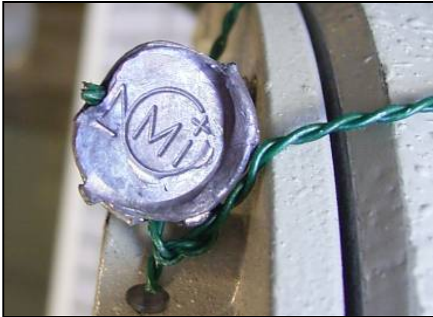
Figure 42: NMI Lead Seal - Typical
