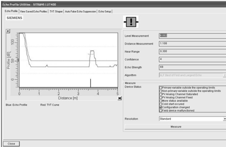
Click on the Measure button to reload the profile. (Select Standard Resolution to update the profile faster. Detailed Resolution uploads all data points.)
