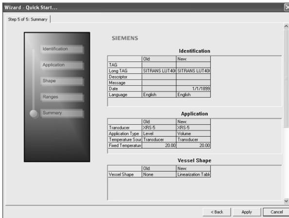
Configuration via AMS Device Manager Quick Start Wizard for a Volume application with a complex vessel shape is now complete.
