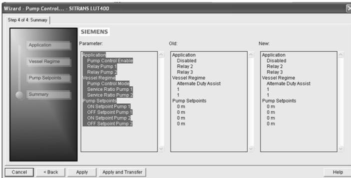
Pump configuration via PDM Pump Control Wizard is now complete.
