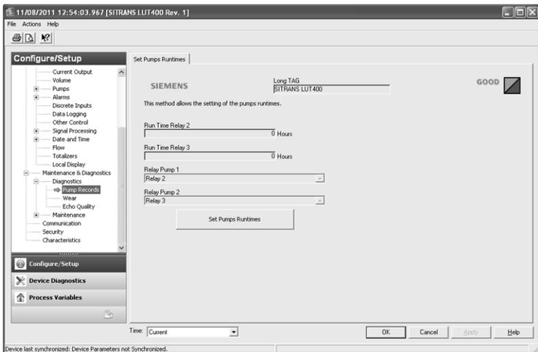
Navigate to **Configure/Setup > Maintenance & Diagnostics** for access to:
