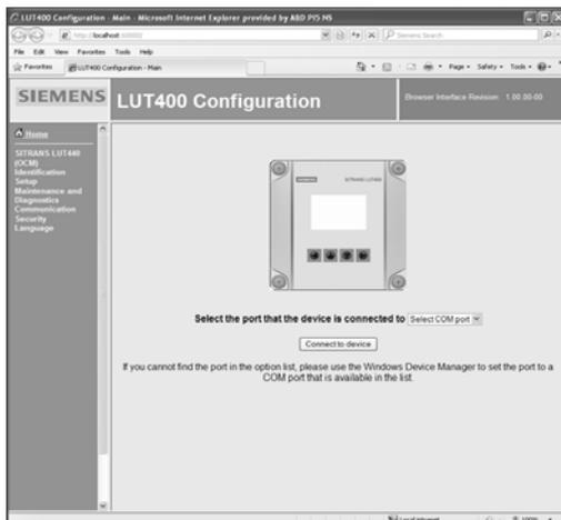
Select the COMPORT that the device is connected to on your computer from the drop-down box. (This is the COMPORT number noted above in step 2 of *Communication port setting*.) The
