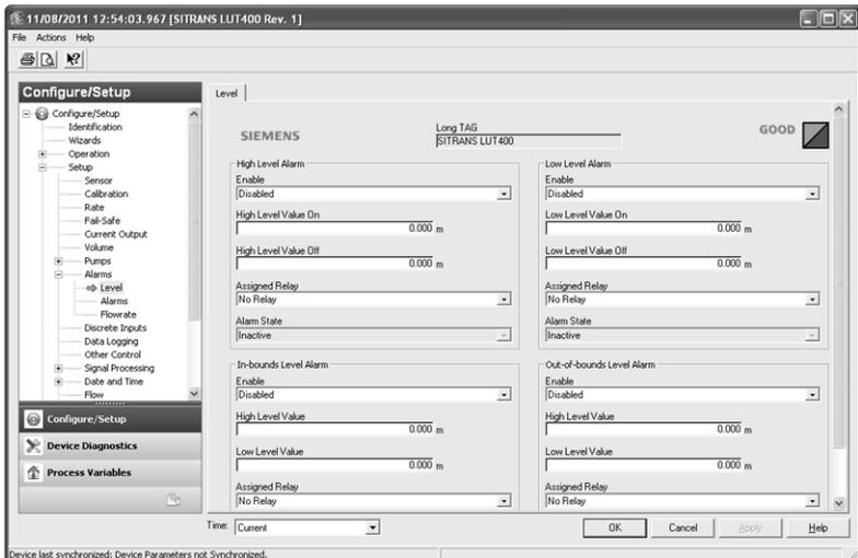
Navigate to **Configure/Setup > Setup > Alarms** for access to:
