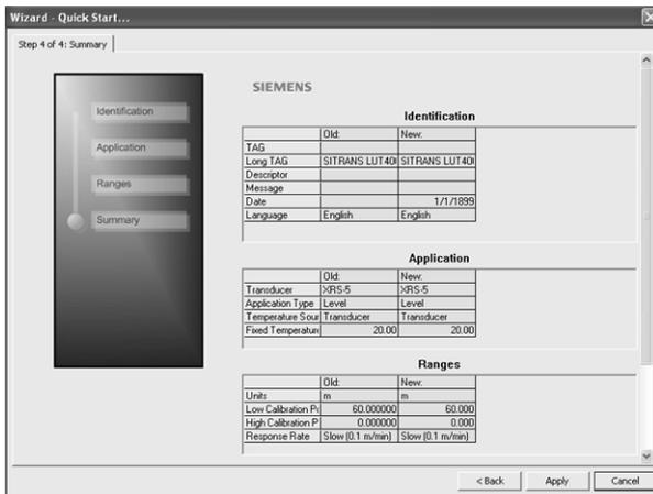
Configuration via the AMS Device Manager Quick Start Wizard for a Level application is now complete.
