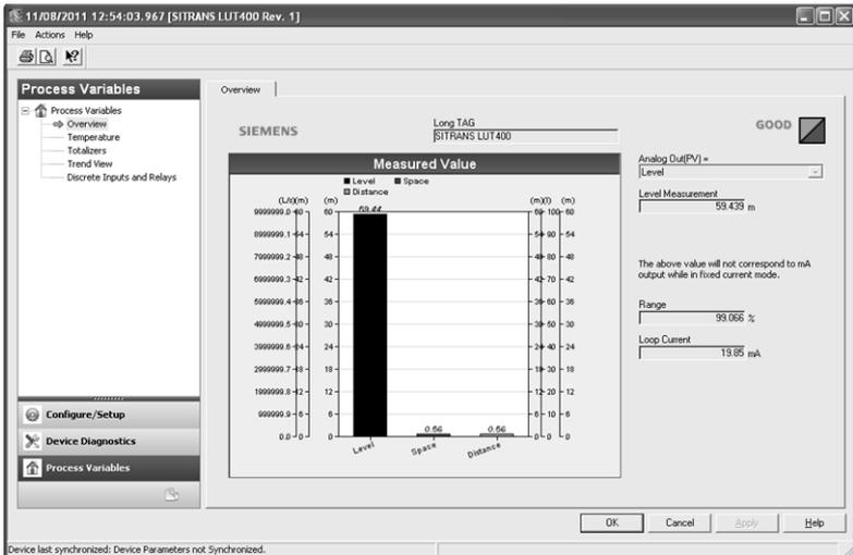
Click on **Process Variables** at the bottom of the navigation window for access to:
