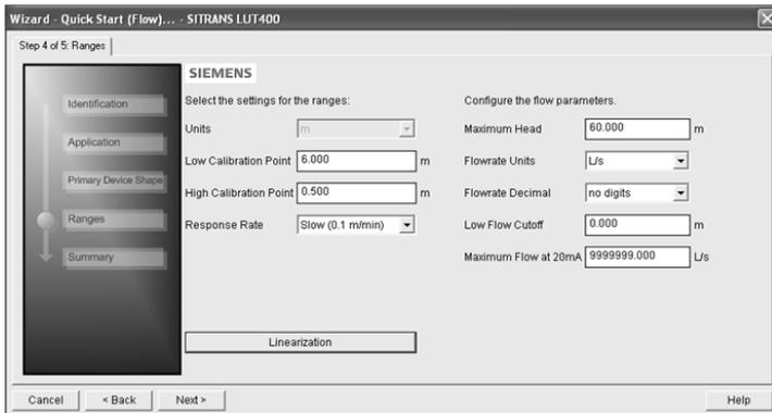
2. If PMD selected in Step 3 was **Universal Head Flow**, the Linearization button will appear in Step 4. Click on **Linearization** to set Head and Flow Breakpoints, then click **OK** to return to the Step 4.
