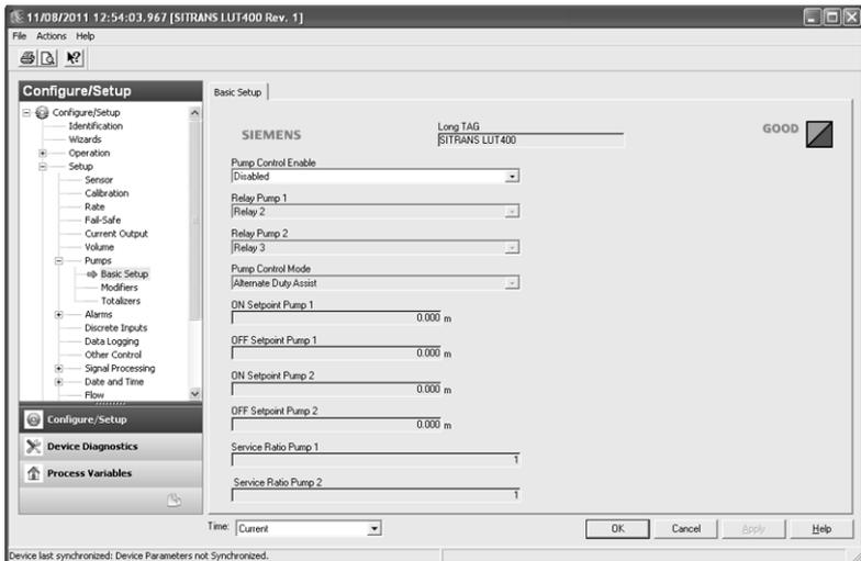
Navigate to **Configure/Setup > Setup > Pumps** for access to:
