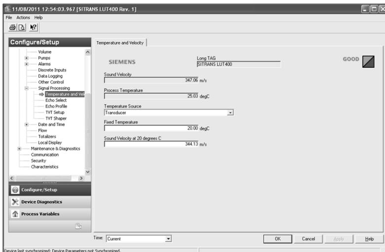
Navigate to **Configure/Setup > Setup > Signal Processing** for access to:
