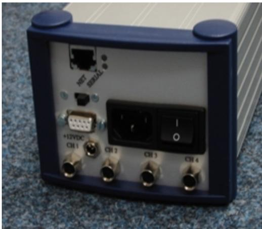
Instruments are delivered with connecting cable (PC connection), line power cable and 12VDC cable.
