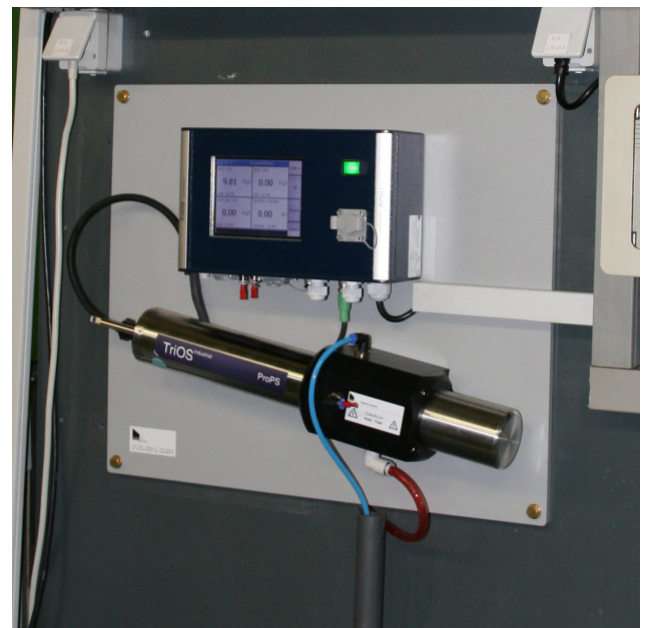
TriBox2 used as a raw water monitoring tool (together with a ProPS sensor) at a drinking water supply
