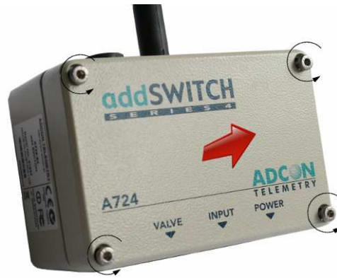
Figure 3. Removing the addSWITCH Lid
