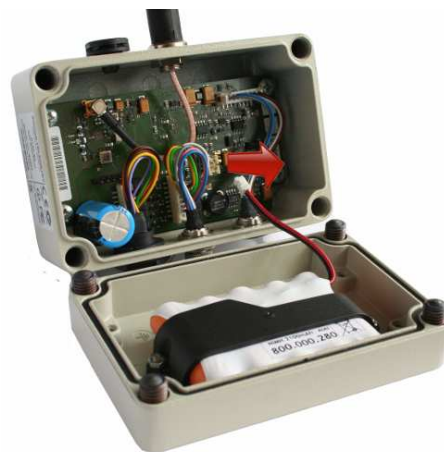
Figure 4. Unplugging the PCB Connector
