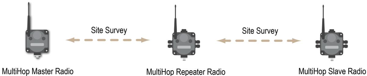
Other radios bound within the same network remain synchronized to the network, but are blocked from sending data while the site survey is running. The site survey analyzes the signal strength between the selected child and its parent radio only. Disable site survey on one radio before initiating it from another.
