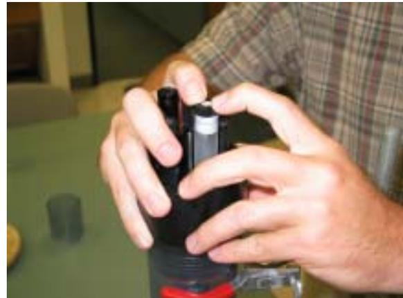
As you screw the sleeve into place, the excess electrolyte is forced out of the sleeve through the reference electrode junction (the white, porous circle at the end of the sleeve). This not only purges bubbles from the electrolyte, but also cleans nasty stuff out of the junction.
