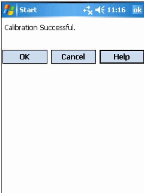
Manta2, Calibrate, SpCond us/cm menu after Sensor Response Factor Y to accept for 2 seconds then returns to Main screen.
