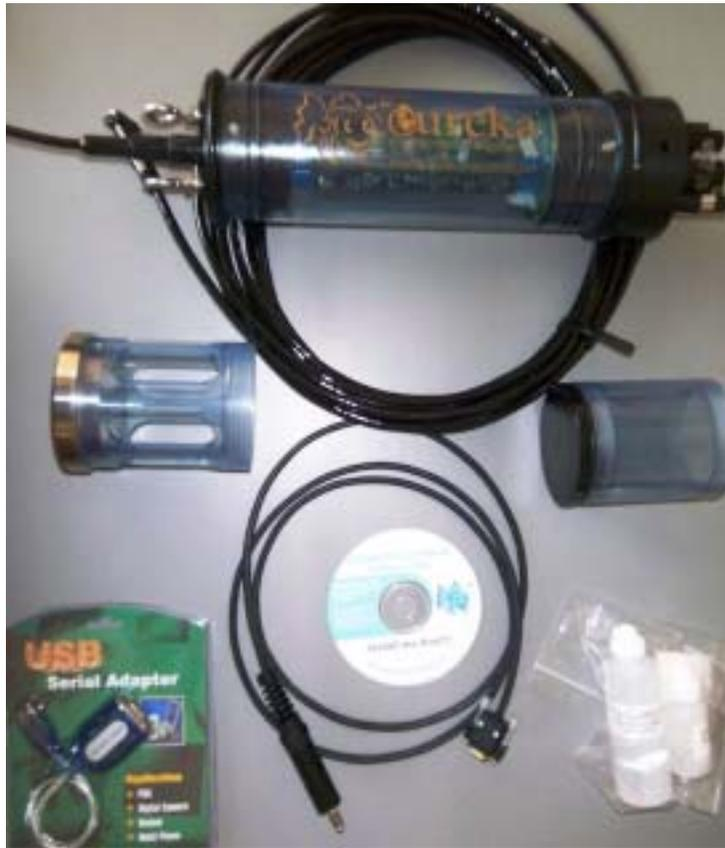
Clockwise from the top: Manta 2 and its underwater cable, storage/calibration cup, maintenance kit, software disc and data cable, USB adapter, weighted sensor guard.
