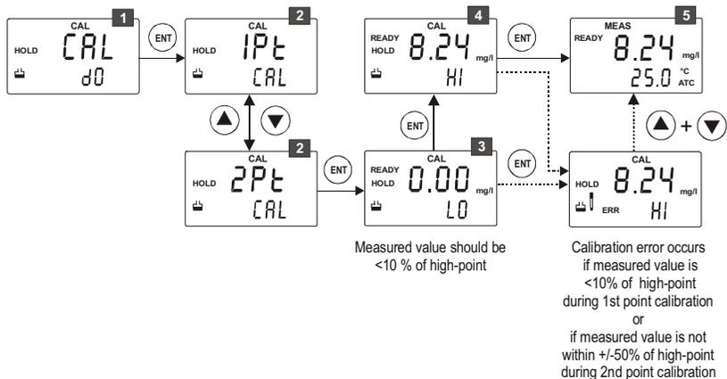
**1** From measurement mode **press CAL key** to enter calibration mode as described in section 4.1. The LCD shows 'CAL Do'. **Press ENT key** to begin first calibration point.
