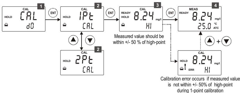
**1** From measurement mode **press CAL key** to enter calibration mode as described in section 4.1. The LCD shows 'CAL Do'. **Press ENT key** to begin calibration.
