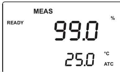
The mode indicator '**MEAS**' at the top of the display indicates that the Transmitter is in Measurement mode. The upper alpha-numerical display shows the measured dissolved oxygen value, while the lower display shows the temperature value. The indicator "%", "ppm" or "mg/l" at the upper right side of the display indicates the current measurement mode. (Refer section 5.2 for switching measurement modes)
