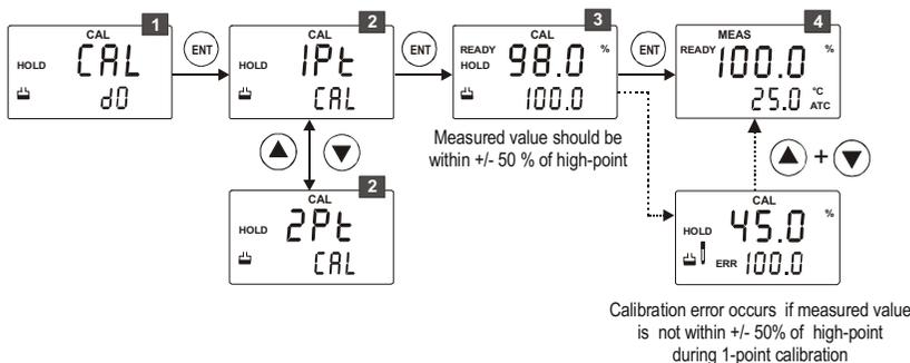
**1** From measurement mode **press CAL key** to enter calibration mode as described in section 4.1. The LCD shows 'CAL Do'. **Press ENT key** to begin first calibration point.
