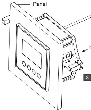
**4** Insert threaded rods through catch until DO Transmitter is held against panel
