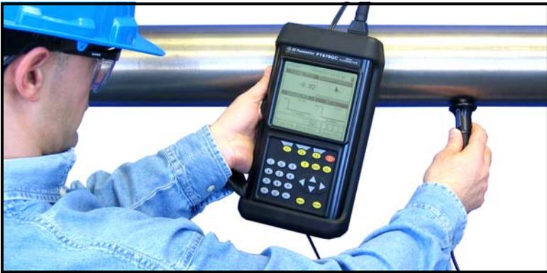
**Figure 9-4: PT878GC Thickness Gauge in Operation**
