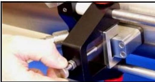
**Figure 3-11: Installing the First Transducer**
