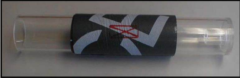
**Figure 3-24: DMP-1 Material with Transducer Footprint Traced**
