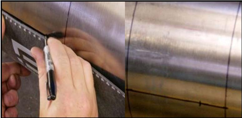
**Figure 3-15: Marking the 9 o'Clock Position**
