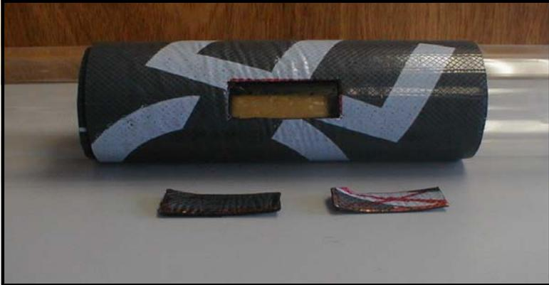
**Figure 3-25: DMP-1 Material with Transducer Footprint Cut Out**
