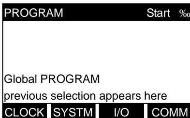
Press the [◆] and [∅] keys and a function key [F1]-[F4] to select the desired submenu. From this screen, press [EXIT] to return to the initial *User Program* screen shown on page 1-8.
