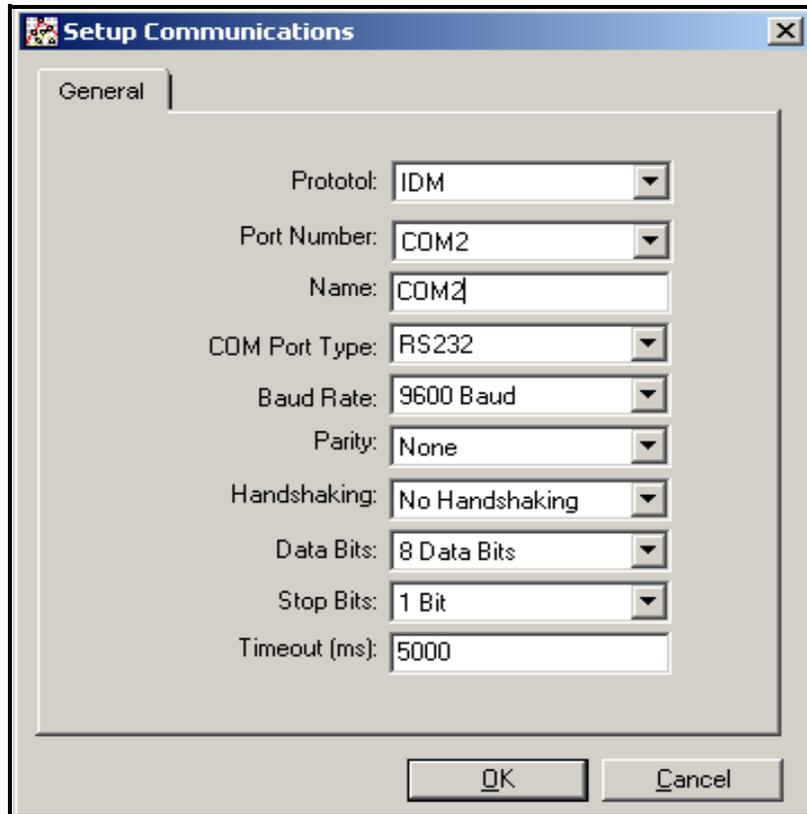
Figure 19: Setup Communications Screen
