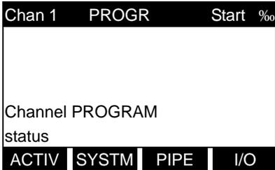
Press the [◆] and [Ø] keys and a function key [F1]-[F4] to select the desired submenu. From this screen, press [EXIT] to return to the initial *User Program* screen shown on page 1-8.
