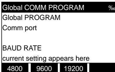
To change the baud rate, press the [Ø] key until the desired baud rate appears on the option bar, and then press the appropriate [F<sub>x</sub>] function key.
