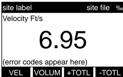
Use the [F1]-[F4], [◆] and [Ø] keys to select the desired display parameter option. Refer to Table 27 on page 56 for a complete description of the available options.
