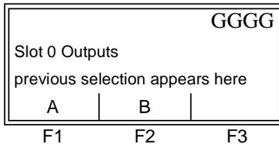
Press [F1] to set up output A or press [F2] to set up output B.
