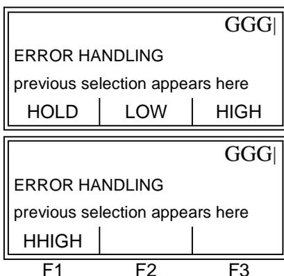
Use the [◀] and [▶] keys to access the options shown. Press the [F $\times$ ] key under the desired error response option.
