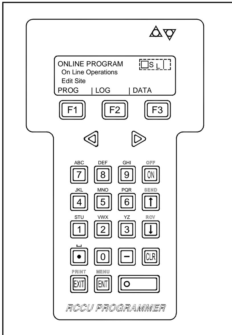
**Figure 1-1: The RCCU Keypad**
