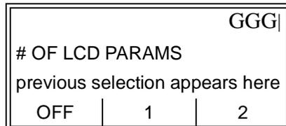
Press the [Fx] key under the desired number of parameters to be sequentially displayed.
