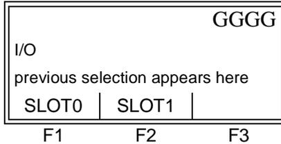
Press the [F $x$ ] key under the desired slot to program the I/O functions in that slot.
