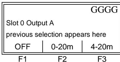
Press [F1] to disable output A and return to the I/O prompt, or press [F2]-[F3] to specify the desired range for output A.
