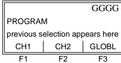
Press the [Fx] under GLOBL to select it. (Note that the CH2 option does not appear for a one-channel meter.)
