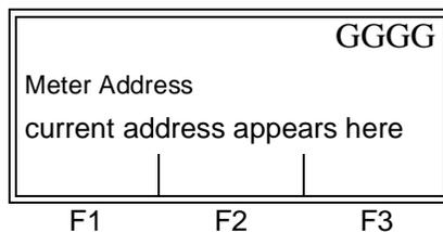
Enter a meter address number between 1 and 254 and press [ENT]. The default number is 1.
