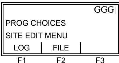
(These additional options only appear if a data logging option card is installed in Slot 2. To access, press the [◀] or [▶] keys.)
