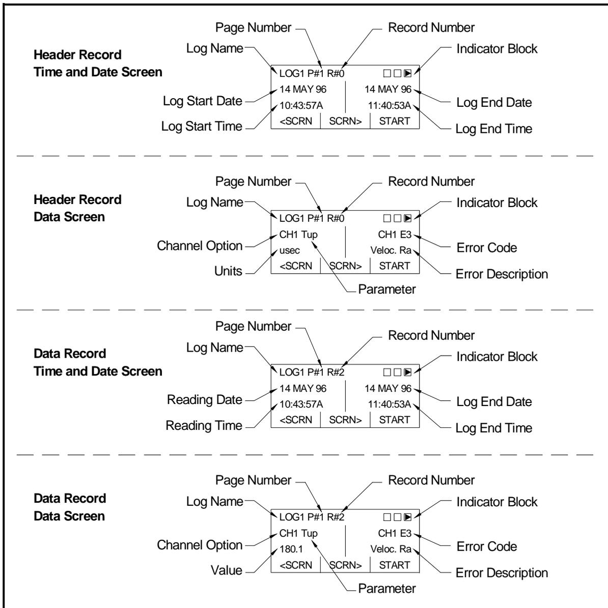
Figure 3-2: RCCU Log Display Screens
