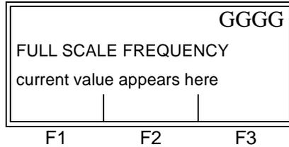
Enter a value between 1 and 10,000 for the frequency at full scale and press [ENT].
