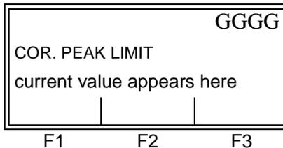
Press [ENT] to accept the current COR. PEAK LIMIT value or enter a new value and press [ENT].
