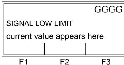
Press [ENT] to accept the current SIGNAL LOW LIMIT value or enter a new value and press [ENT].
