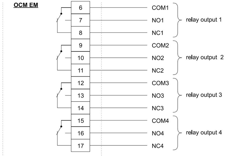
Figure 29. Wiring Diagram of relay outputs
