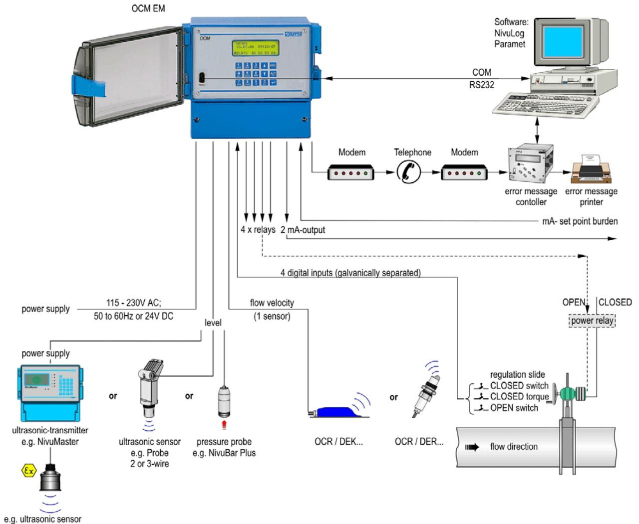
Figure 3. Combination possibilities of the measurement technique
