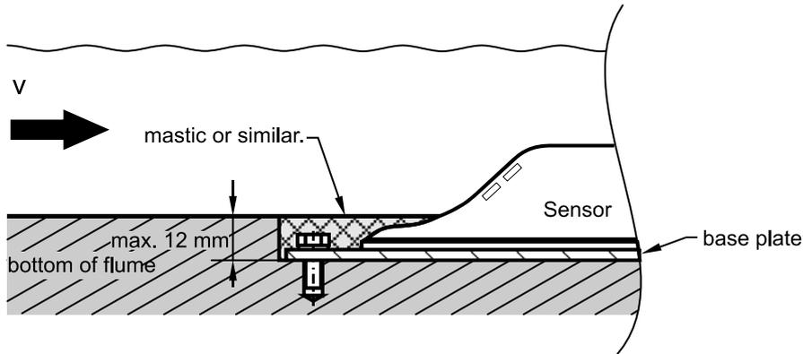
Figure 13. Mounting Suggestion for Wedge (mouse) Sensor Under the Floor
