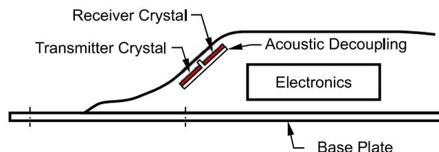
Figure. 4. Construction flow velocity sensor
