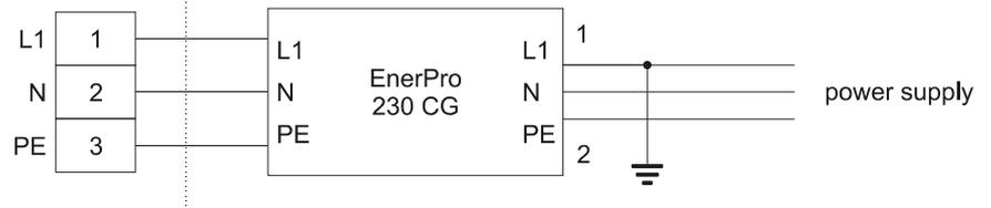
Figure 31. Connection Overvoltage Protection Power Supply
