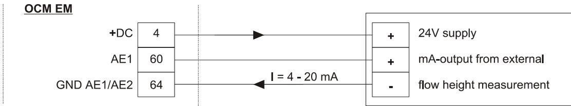
Figure 27. External 3- wire Sensor for Level Measurement
