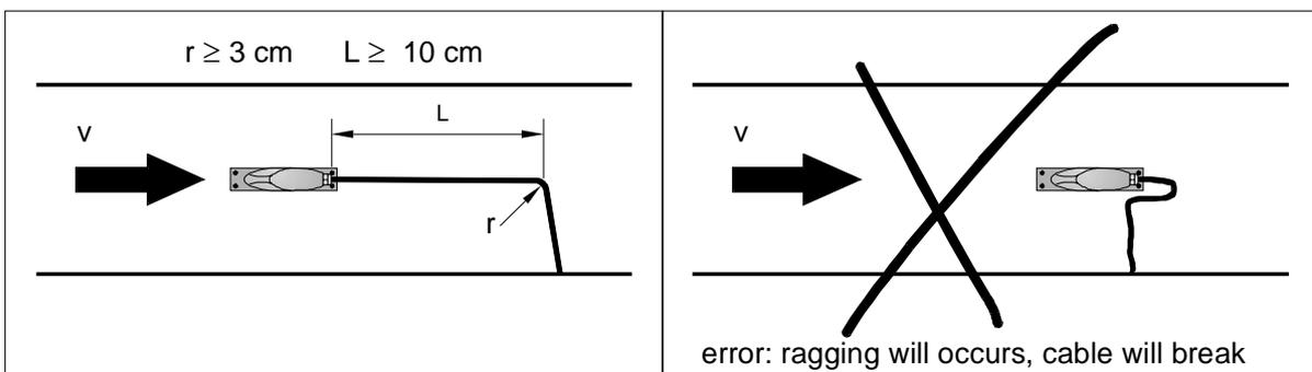
Figure 16. Mounting Notes for Flow Velocity Sensors
