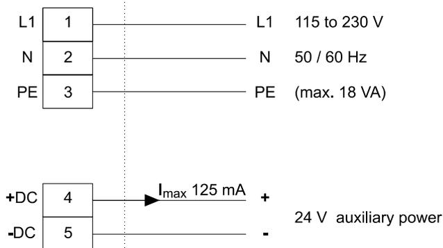
Figure 9. connection OCM EM, Type „AC“
