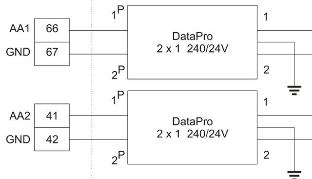
Figure 33. Connection Overvoltage Protection Analog Output
