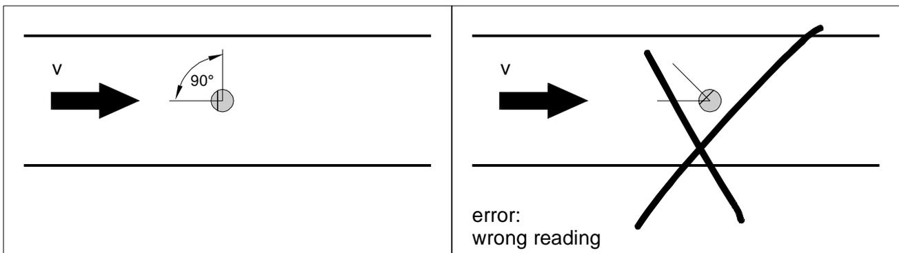
Figure 17. Mounting Notes for Pipe Sensors
