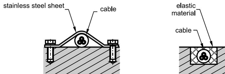
Figure 14. Mounting Suggestion for Laying Cable
