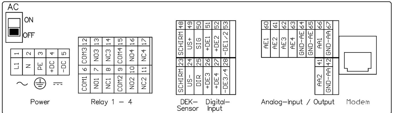
Figure 7. connection plan of the OCM EM
