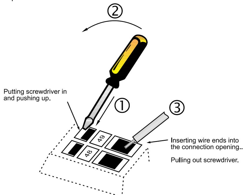
Figure 6. connecting the wires in Cage train spring clips
