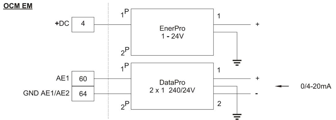
Figure 35. Connection Overvoltage Protection Level Sensor 3-Wire
