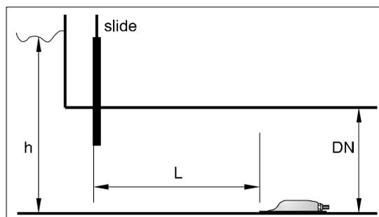
Figure 24. Require Distance behind Slide Gates
