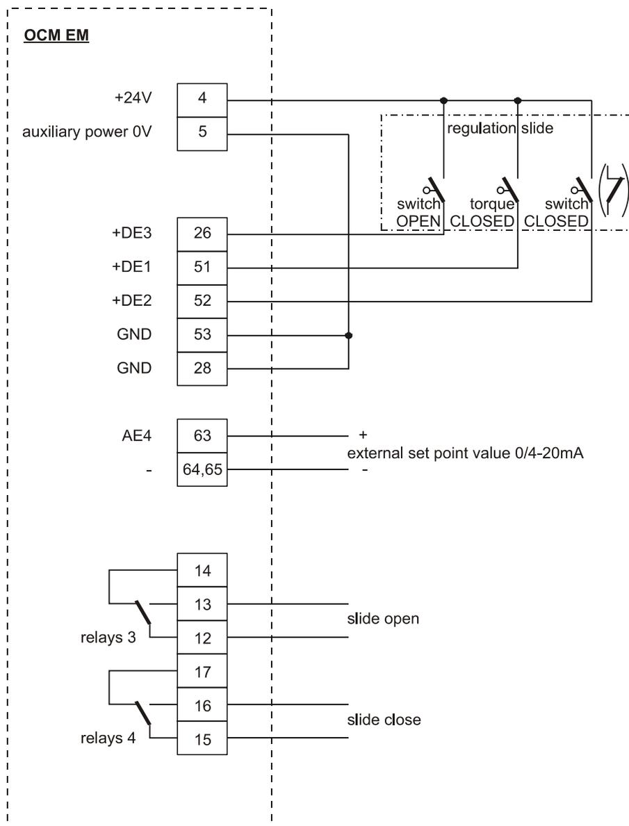
**Note:** Relay 1 and 2 are not suitable to control the regulation slide.
