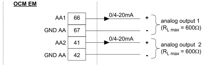
Figure 28. Wiring Diagram of analog outputs
