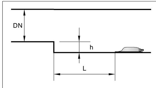
Figure 22. Required distance from a step or drop
