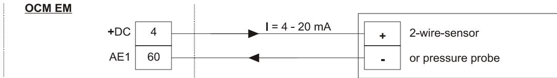
Figure 34. Connection Overvoltage Protection Level Sensor 2-Wire
