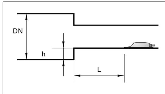
Figure 20. Require Distance after Profile changes
