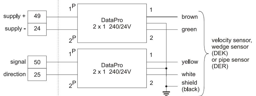
Figure 32. Connection Overvoltage Protection Velocity Sensor
