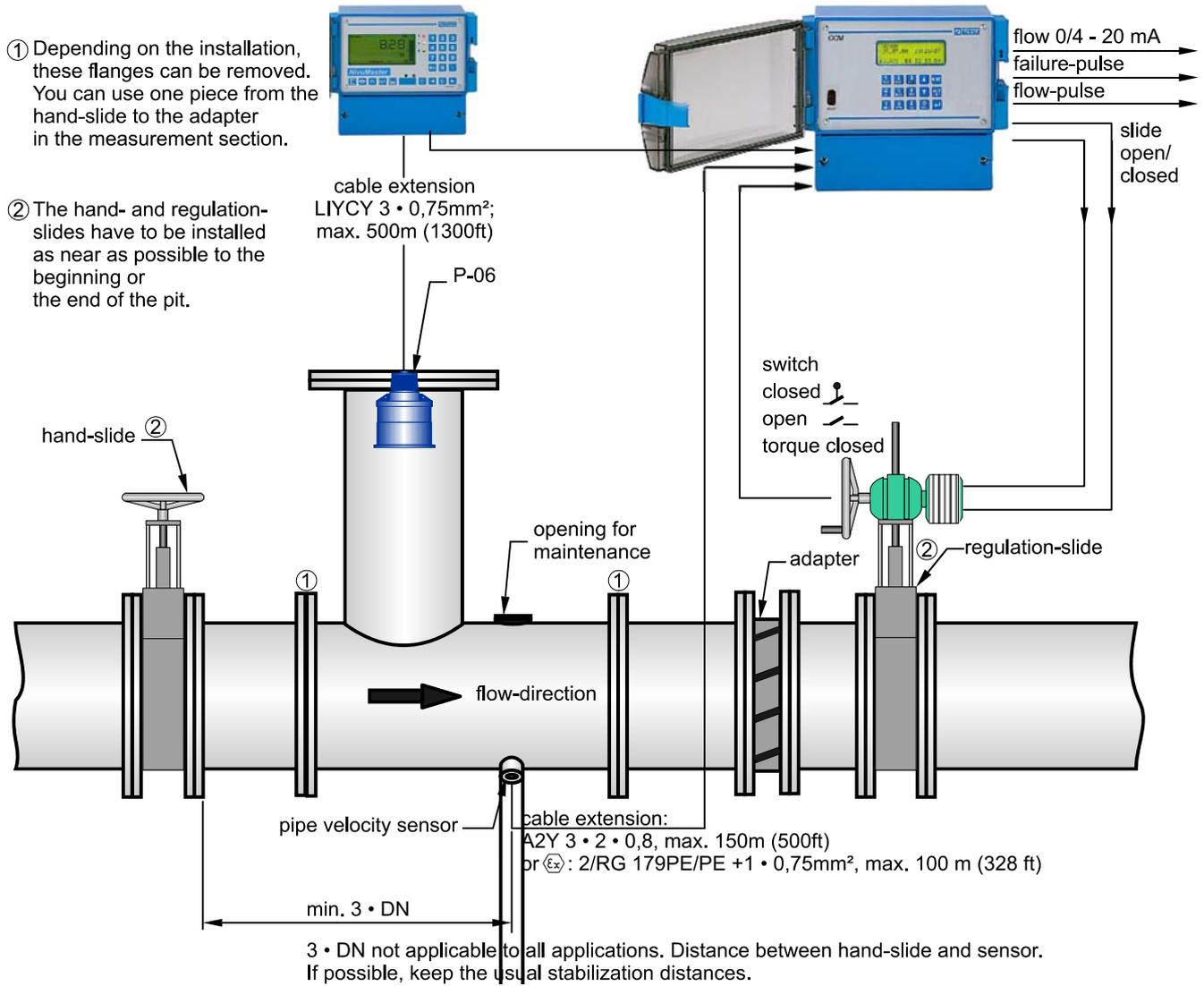
Figure 19. Construction measure-and controlled section
