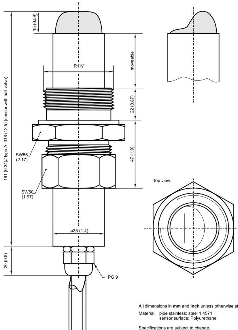
Figure 12. Drawing Insertion Sensor
