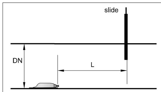
Figure 23. Require Distance in Front of Slide Gates
