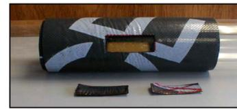
8. Once again remove the transducers and clamping fixture. Use a knife to cut out the transducer shape and peel the dampening material from the pipe.
