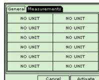
9. You now need to set the measurements to be recorded. Scroll up to the General tab and across to the 'Measurements' tab. Press [ENTER] to go to this tab.
