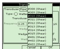
2. Work through the transducer options selecting the appropriate options from the drop down menus, or manually type in the correct selection (if a box is greyed out you do not need to enter a selection for this parameter). *Wedge temperature is typically half way between the pipe and air temperatures.*
