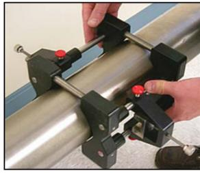
**Note:** Each half of the fixture has a measuring scale. Ensure that the scales are on the same side of the fixture with zero at the same origin.
