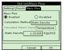
3. If you have selected "Enable" Mass Flow the following prompt will appear asking for the calculated method. Three options are available: static density, saturated steam and steam. Press [ENTER] to open the drop-down menu. Scroll to the appropriate method for your application and press [ENTER] to confirm the entry.
