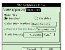
8. The next prompt will appear whether you have selected an active or fixed temperature value. The desired input needs to be entered. Scroll from the Temperature text box to the Input menu and press [ENTER] to open the drop down menu. Scroll to input A or B and press [ENTER] to confirm the selection.
