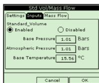
5. The next prompt will appear whether you have selected an active or fixed pressure value. The desired input needs to be entered. Scroll from the Pressure text box to the Input menu and press [ENTER] to open the drop down menu. Scroll to input A or B and press [ENTER] to confirm the selection.
