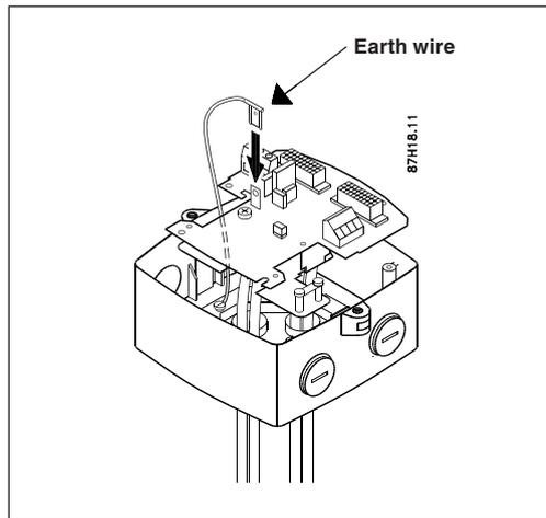
In mains powered units the protective earth wire must be connected to the PE
