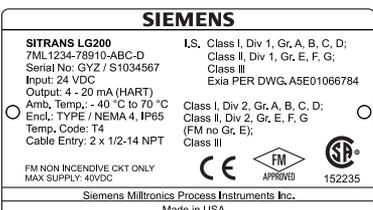
An intrinsically safe (IS) installation potentially has flammable media present. An approved IS barrier must be installed in the non-hazardous (safe) area. Observe electrical data below:
