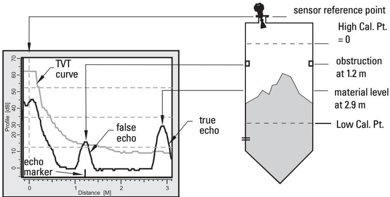
In most cases the material echo is the only one which rises above the default TVT curve. In a vessel with obstructions a large false echo may rise above the default TVT. The Auto False Echo Suppression feature (see below) can be used to screen it out.
