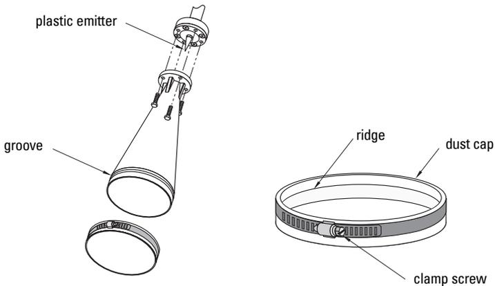
2. Press the cap firmly onto the horn until the ridge inside the cap snaps into position in the groove on the outside of the horn.
