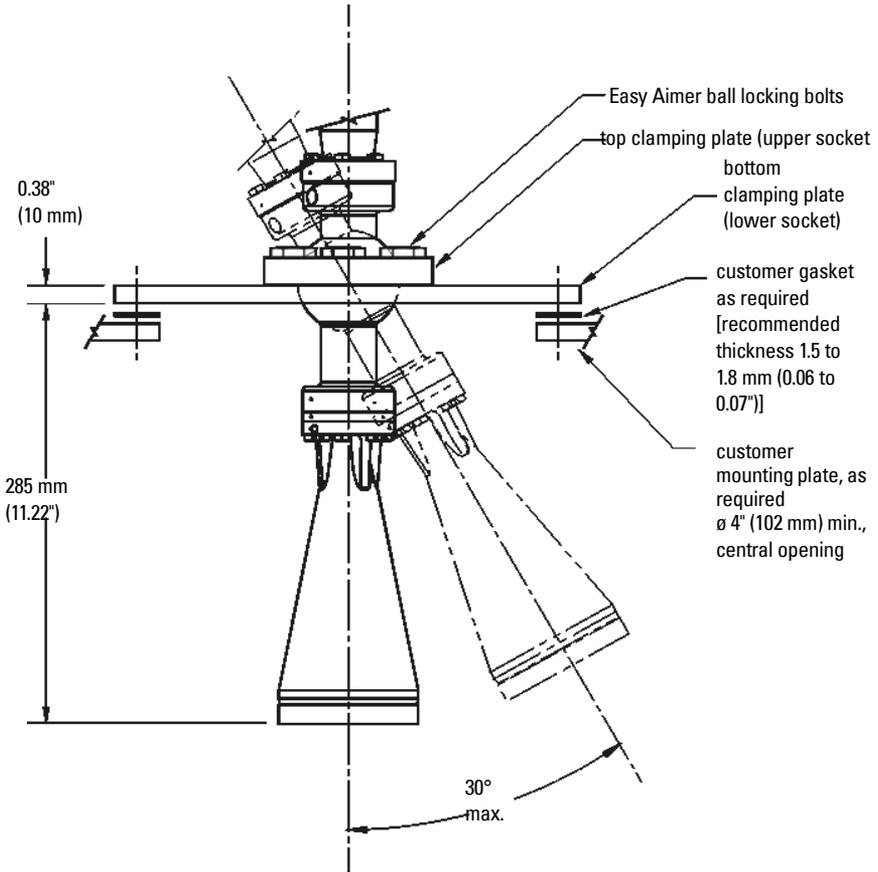
**Note:** When the Easy Aimer ball is loosened, the device is free to tilt to a maximum of 30°.
