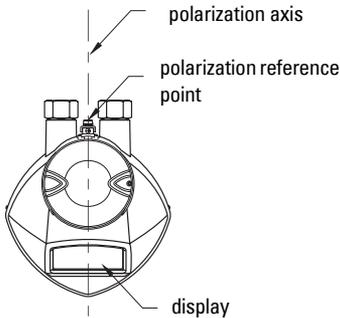
For best results on a vessel with obstructions, orient the front or back of the device toward the obstructions.
