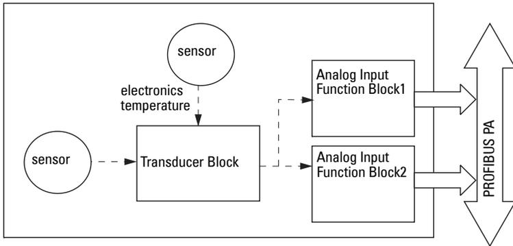
The device is implemented with one Physical Block (PB1), one Level Transducer Block (LTB1), and two Analog Input Function Blocks (AIFB1 and AIFB2).
