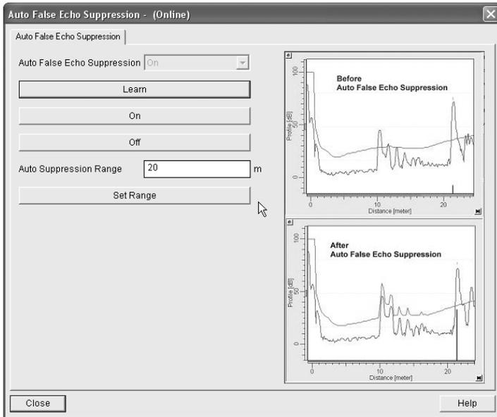
1. Determine **Auto Suppression Range** (the distance within which the learned TVT will replace the default TVT). Measure the actual distance from the antenna reference point to the material surface using a rope or tape measure, and make allowances for the actual location of the LR260. Subtract 2 m (6.56 ft) from this distance, and use the resulting value.
