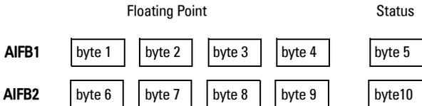
The first 4 bytes are the floating point representation (IEEE) of the variable. The variables are the outputs of the function block. The 5th byte is the status word and the list of possible values is given in the chart below.
