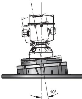
Aiming is not required for signal optimization with 78 GHz frequency.
