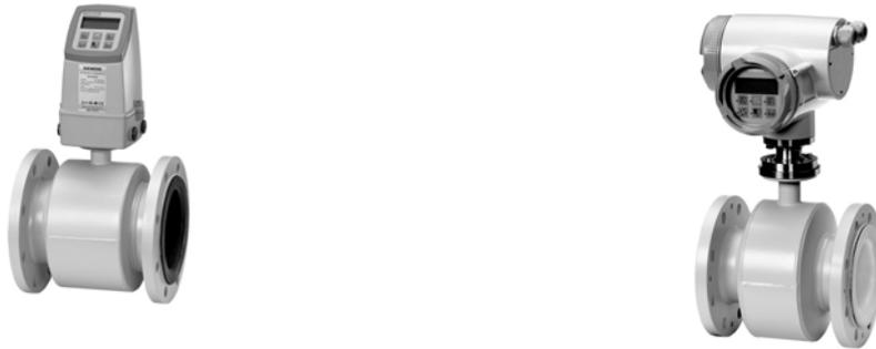
Sensor housing and flanges are designed in carbon steel (ASTM A 105) and terminal box in fibre glass reinforced polyamide or optionally in stainless steel (AISI 316). Measuring pipe is made of stainless steel (AISI 304) while liners and electrodes are available in various material, which makes the sensor highly resistant to a wide range of chemicals.
