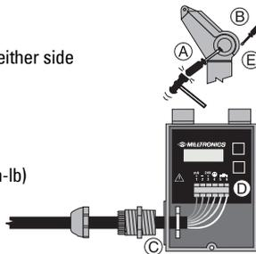
**Note:** Non-metallic enclosure does not provide grounding between conduit connections. The use of approved watertight conduit hubs/glands is required for Type 4X / NEMA 4X / IP65 (outdoor) applications.
