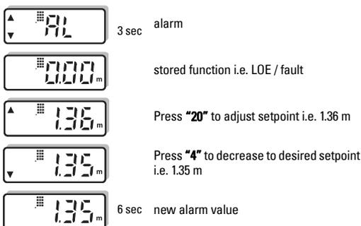
**Note:** For faster scrolling, hold the key depressed during the setpoint adjustment and release when the desired value is obtained.
