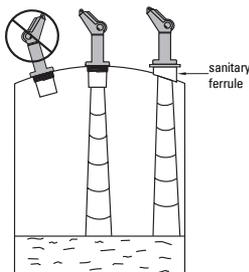
The Probe's sound path should not intersect the fill path rough walls, seams, rungs, etc
