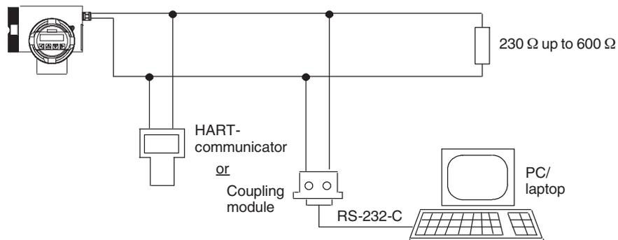
Figure 6-2 System integration via HART
