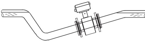
Figure 4-5 Installation in a constantly filled pipe
