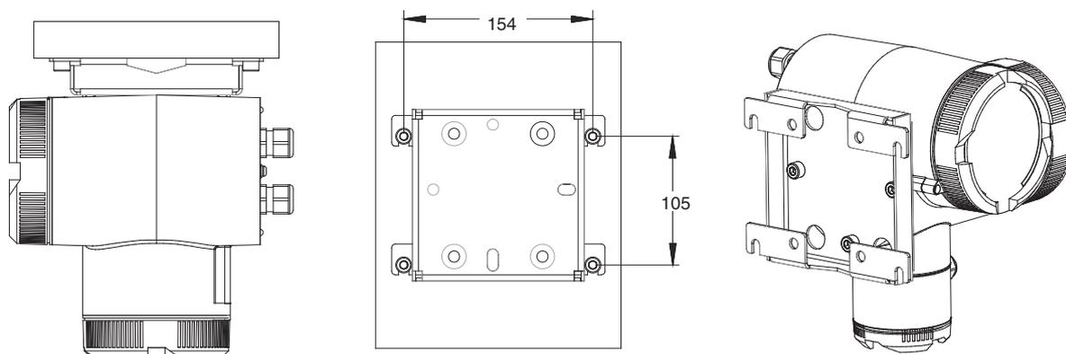
Wall mounting with assembly bracket
