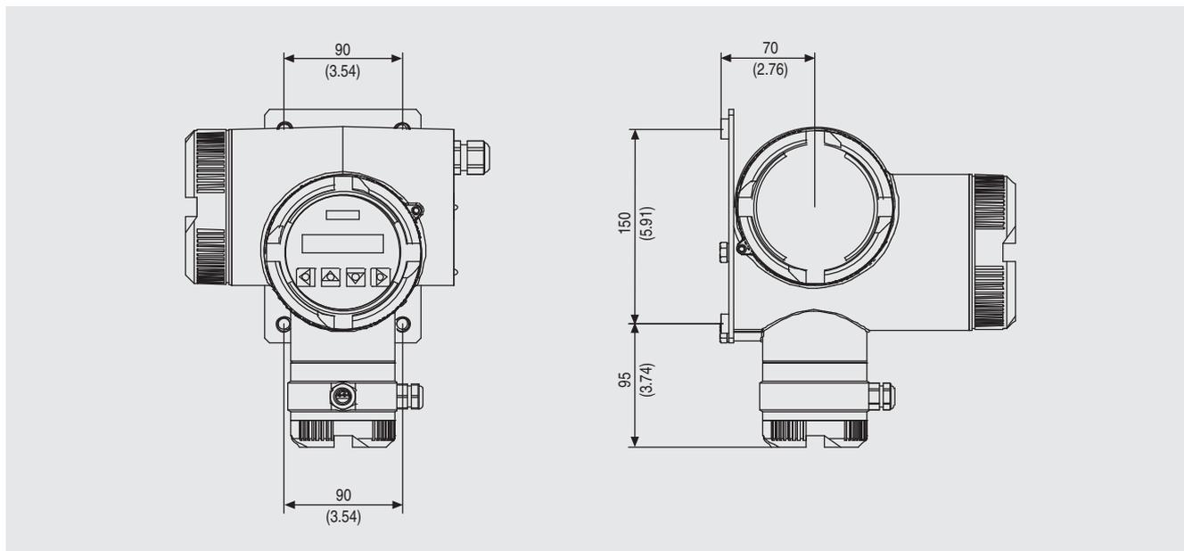
Figure 10-1 SITRANS FM Transmag 2 transmitter (remote design) with standard mounting plate
