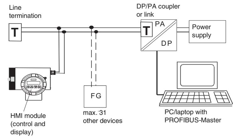
Figure 6-3 System integration via Profibus
