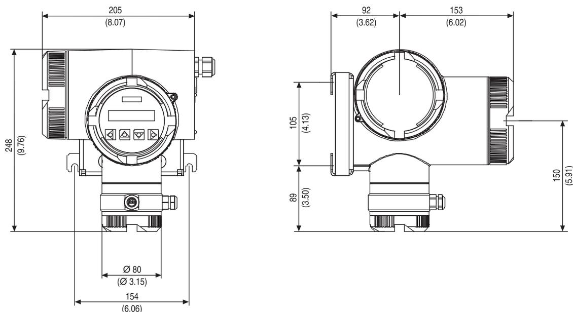
Figure 10-2 SITRANS FM Transmag 2 transmitter (remote design) with optional mounting plate for pipeline mounting
