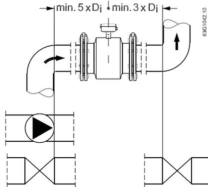
Figure 4-2 Installation between pipe elbows, valves and pumps
