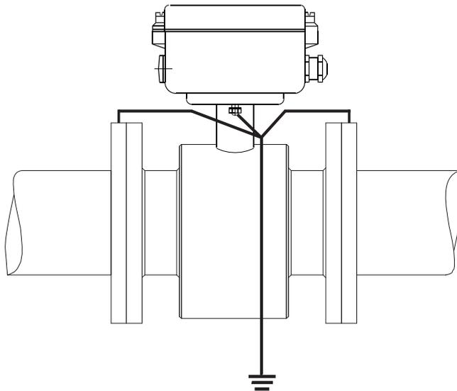
Figure 4-7 Reference potential in electrically conductive pipes
