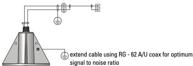
**Note:** Grounding transducer as shown is mandatory per safety regulations and for isolation against electrical interference.
