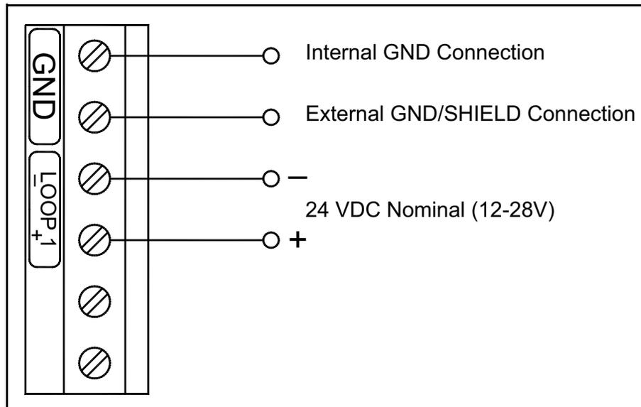
Figure 13: Electrical Connections
