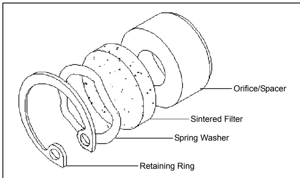
**Figure 16: Filter Components**
