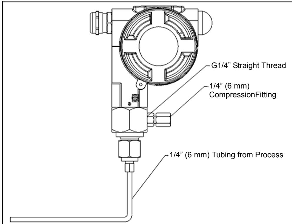
Figure 8: DewPro MMY 30 Remote Wall-Mount Installation with Bypass
