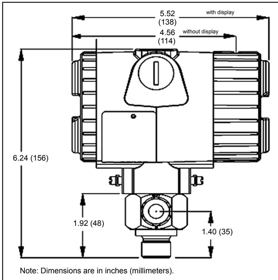
Figure 4: DewPro MMY30 Dimensions with Optional Display/User Interface
