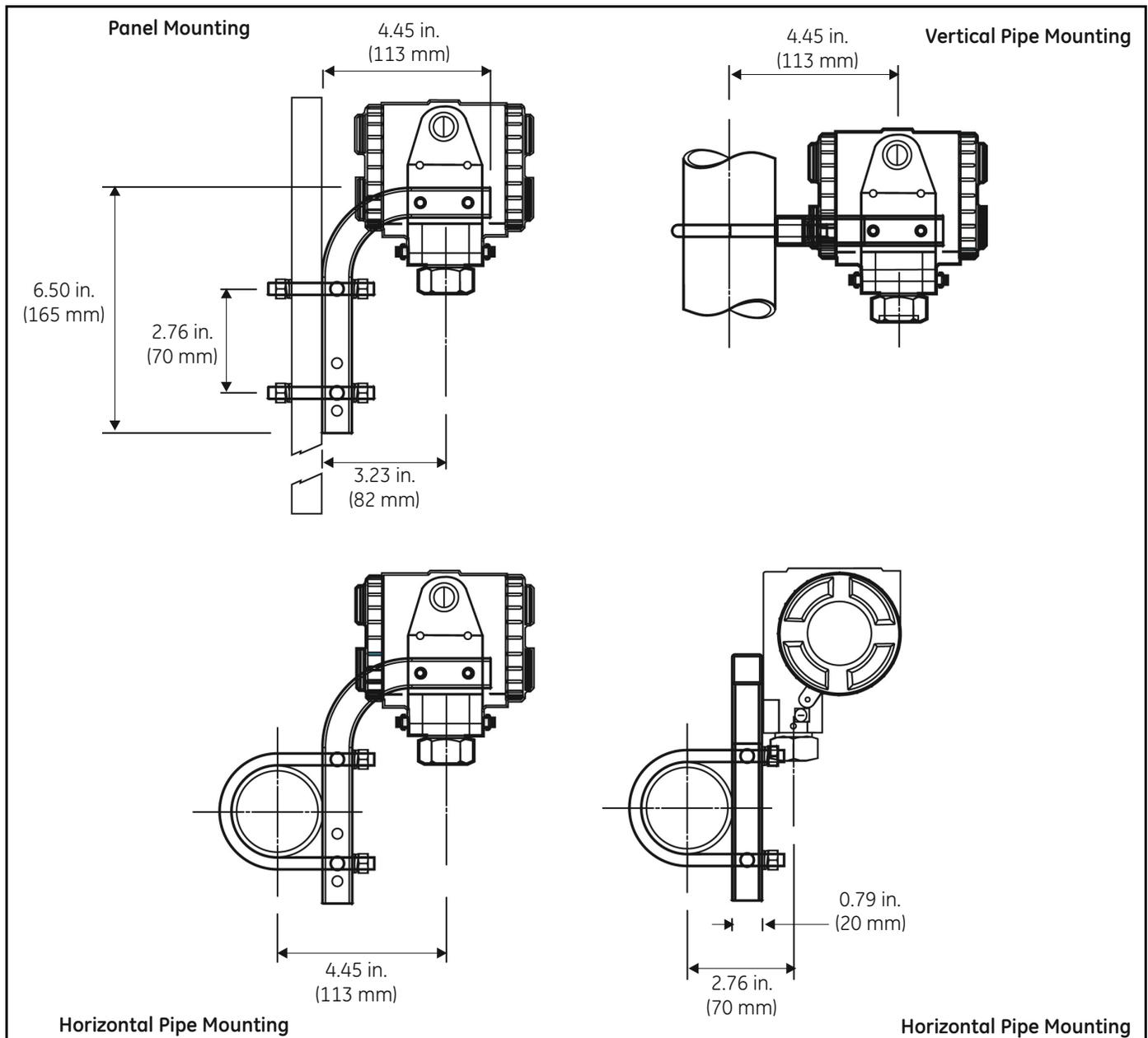
Figure 9: DewPro MMY30 with Various Mounting Brackets
