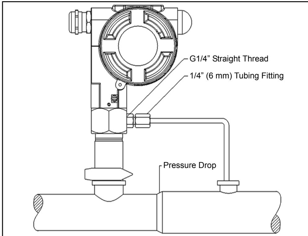
Figure 7: DewPro MMY30 Installation with No Flow Restriction
