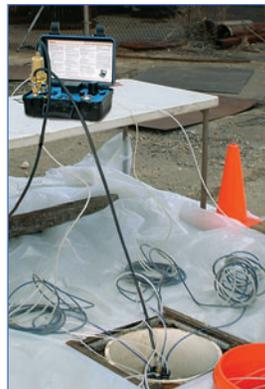
An EPA regulated site in Northeast, USA. This multilevel array allowed a sampling team to purge and sample from 40 monitoring zones across 10 borehole locations in just 4 days. These Waterloo Systems were installed in overburden using preinstalled casing.
