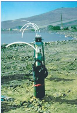
Landfill site over fractured granite, monitored with five Waterloo Systems. Each System comprised of dedicated Double Valve Pumps and Pressure Transducers in 4-6 intervals to depths of 275 feet (84m). The Multi-Purge Manifold allowed the monitoring of 21 zones to be completed in less than 2 days.
