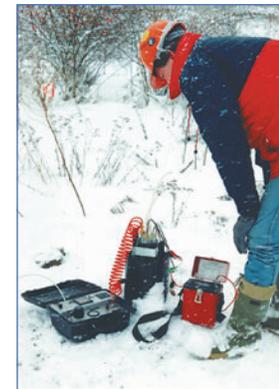
750ft. (230m) Waterloo System installation for a deep tunnel assessment study. Three zones monitored with dedicated Double-Valve Pumps and pressure transducers. Picture shows technician obtaining pressure measurements and groundwater samples with portable readout and pump control unit.
