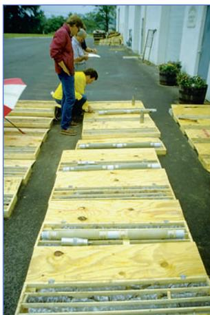
Using core logs to identify placement of Ports and Packers
