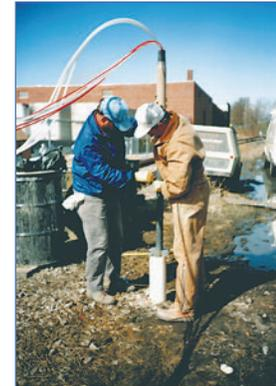
Detailed investigation of PCE delineation in carbonate bedrock. A cost analysis of the 14 Waterloo Systems compared with nested piezometers indicated savings both on the capital costs and on the on-going monitoring.
