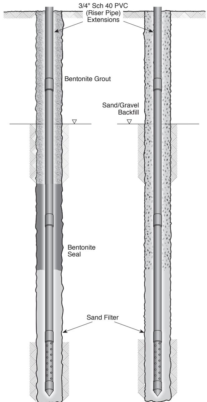
Typical Standpipe Piezometer Installations
