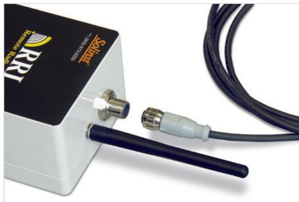
Figure 6-2 External Power Cable Connection
