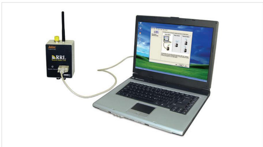
Figure 4-6 RRL Station Connected to a PC
