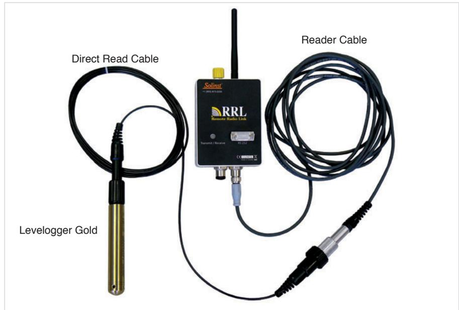
Figure 2-5 Connecting Levelloggers
