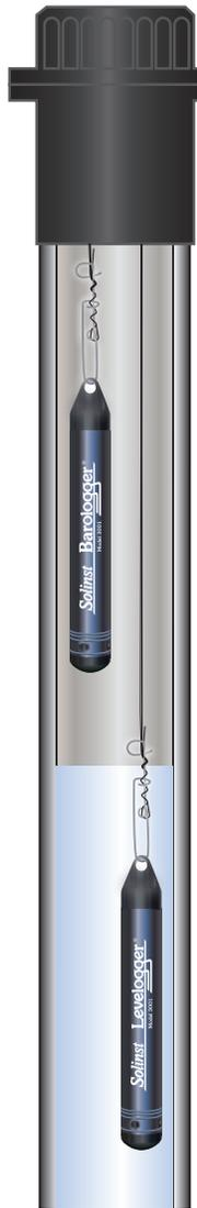
Figure 10-12 Levellogger and Barologger in Well
