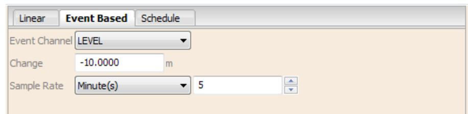
Figure 5-11 Event Based Sampling Setup
