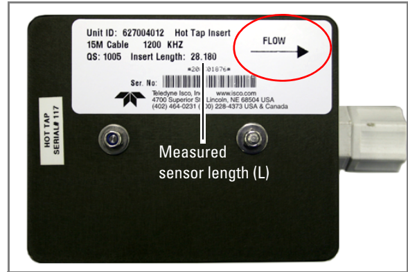
Figure 3: Sensor length and flowstream alignment
