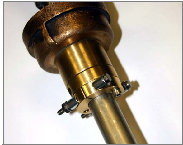
Figure 6: Hot Tap with secondary collar installed
