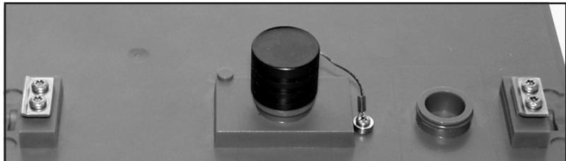
Figure 1-6 Flow Module - Upper connector, capped
