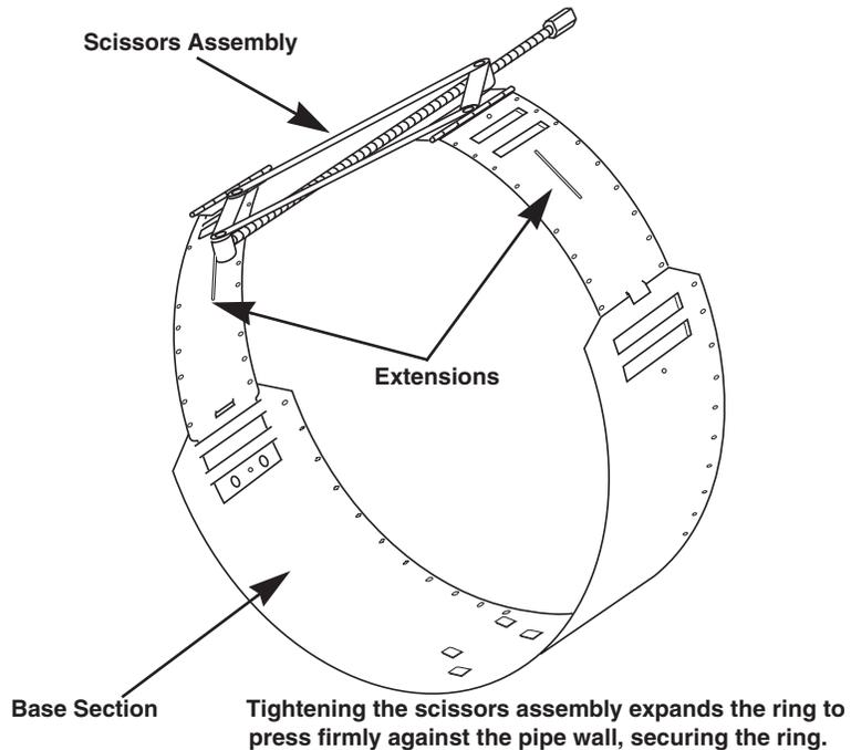
Figure 2-8 Scissors Ring adjustment
