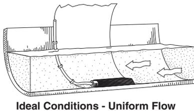
See Section 2.6 for a summary of sensor mounting options for round pipe installations. Sensor installation is discussed in detail in *Iscos Mounting Rings Instruction Manual*. The manual explains how to mount the low profile AV Sensor in flow streams using spring rings, scissors rings, a street level installation tool, and mounting plates.
