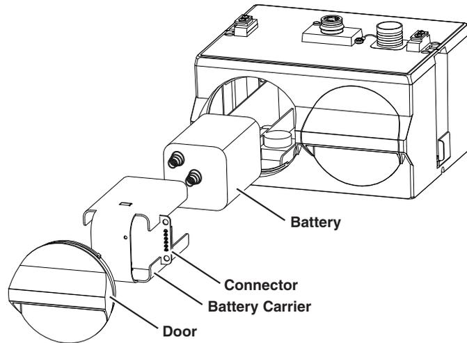
Figure 2-3 Installing a Battery
