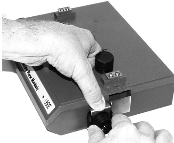
Figure 1-10 Flow Module - preparing the sensor connectors
