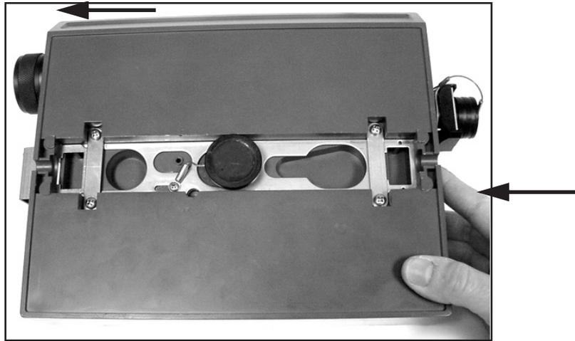
*Figure 1-16 Flow Module - Unlocking the latch*
