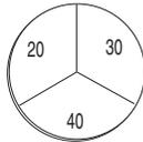
A humidity indicator is mounted inside each battery cap on the Battery Module. The humidity indicators have regions that display 20, 30, and 40 percent humidity levels. Ideally each region should be completely blue. As the desiccant becomes saturated, the humidity levels will increase and the regions turn pink. When the 40 percent region turns pink, the Battery Module is no longer adequately protected and the desiccant must be replaced. Refer to section 5.4 for replacement instructions.
