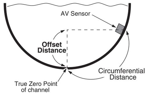
Figure 3-3 Zero Level Offset Measurement
