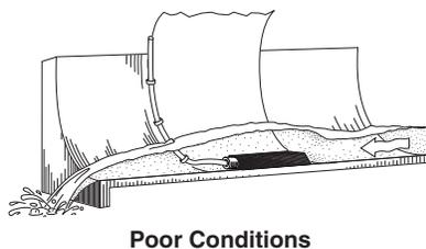
The example in the margin shows a few of these poor conditions. The outfall is drawing down the liquid level and the AV Sensor is disturbing the flow. In this example, the AV Sensor should be moved forward to avoid the drawdown near the outfall.
