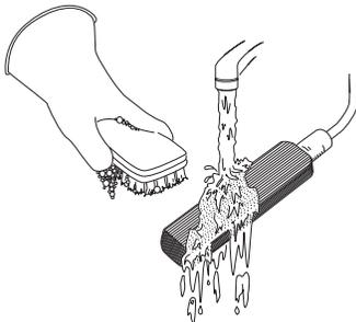
The AV Module case may be cleaned with mild detergent and warm water. Before cleaning the module, ensure that all protective connector caps are in place.
