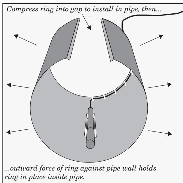
Figure 2-7 Sensor Installed on a Spring Ring
