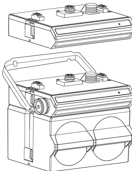
*Figure 2-4 Assembling a system (shown: 2 flow modules with 1 battery module)*
