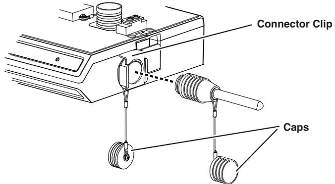
Figure 2-5 Connecting the AV Sensor
