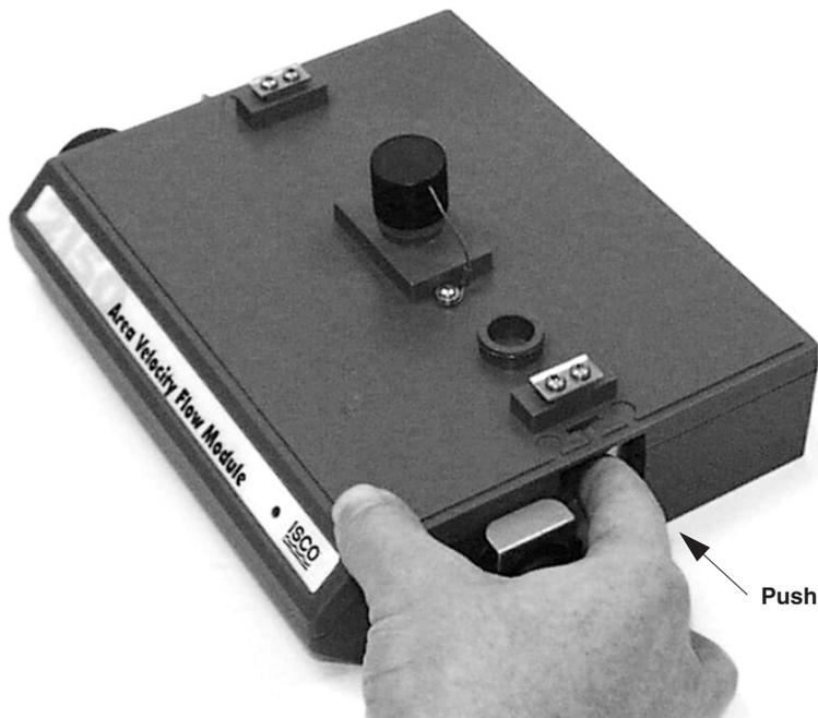
Figure 1-5 Unlocking the Latch
