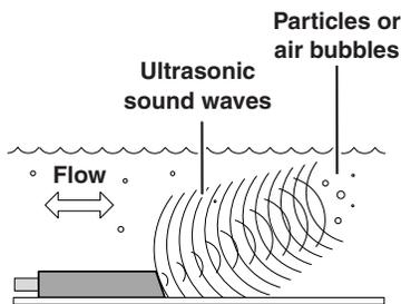
The AV Sensor measures average velocity by using ultrasonic sound waves and the Doppler effect. The Doppler effect states that the frequency of a sound wave (or other wave) passed from one body to another is relative to both their motions. As the two approach each other, the frequency increases; as they move apart, the frequency decreases.
