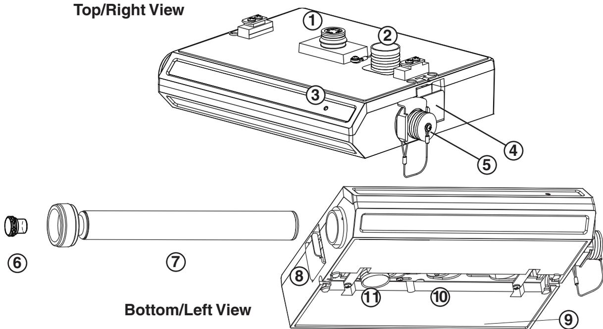
Figure 1-1 Controls, connectors, and indicators – 2150 Flow Module
