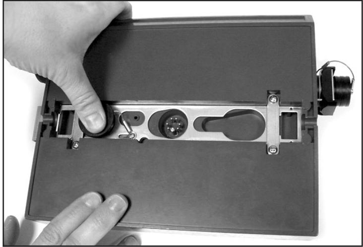
*Figure 1-18 Flow Module - Pushing plug into holder*
