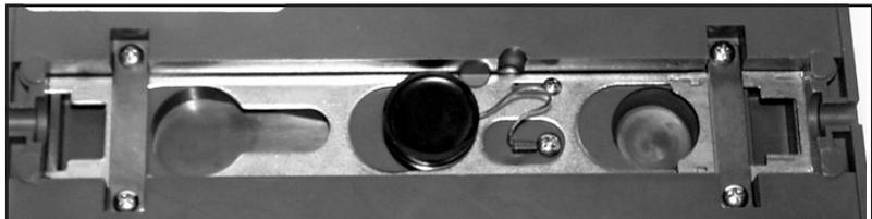
Figure 1-8 Flow Module - Lower connector, plugged
