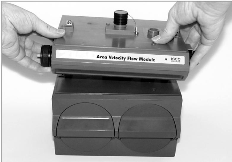
*Figure 1-21 Aligning the modules*
