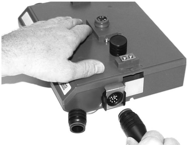
Figure 1-11 Flow Module - connecting the sensor
