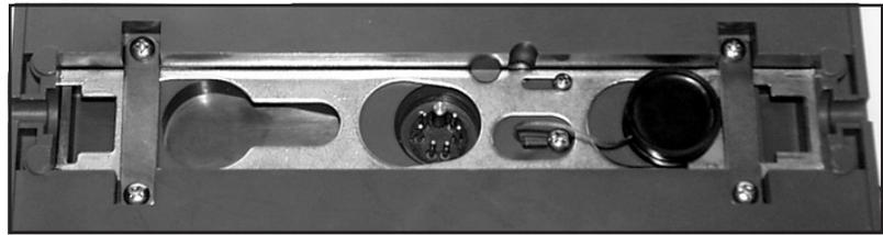
Figure 1-9 Flow Module - Lower connector, unplugged
