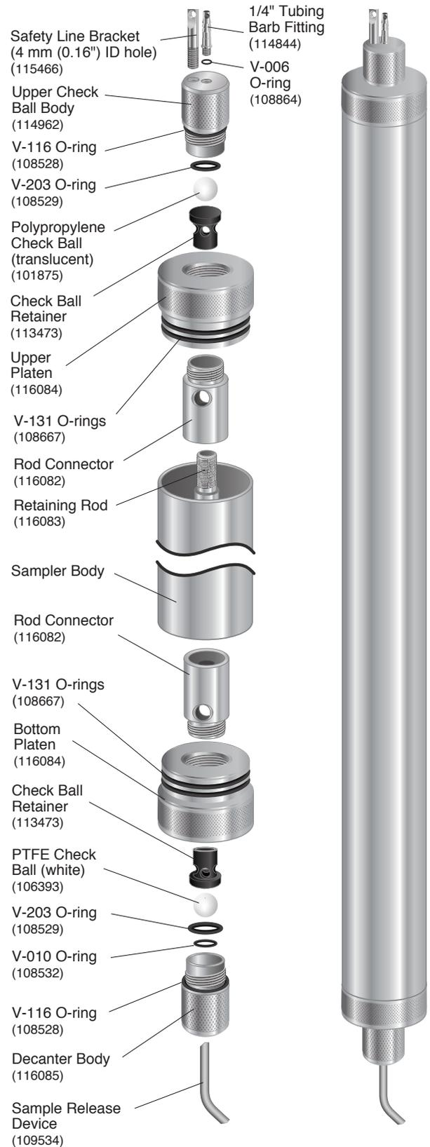
*Model 425 Mk3 2" x 2 ft. Discrete Interval Sampler (115012)*
