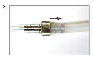
Figure 2-8 Attaching the suction line to the pump tubing
