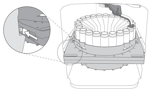
Figure 2-4 The 24-bottle rack is held in place by a latch on the left side
