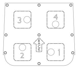
Figure 2-6 Four-bottle, 20L locating base: Bottle mouth placement
