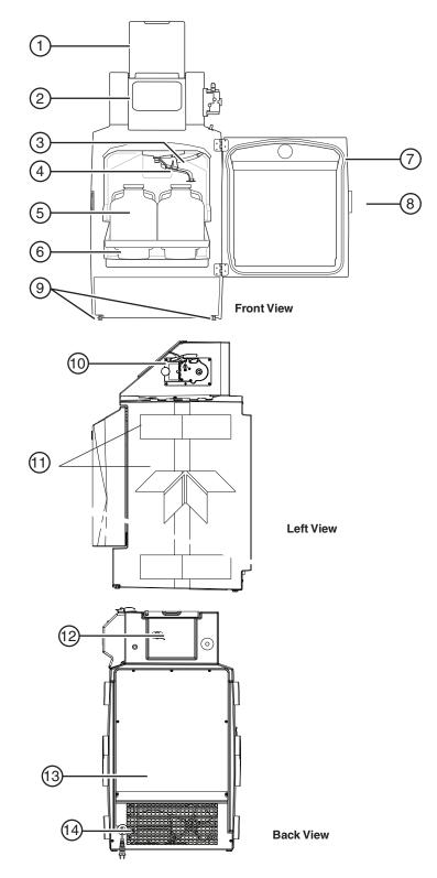
Figure 1-1 5800 Sampler features
