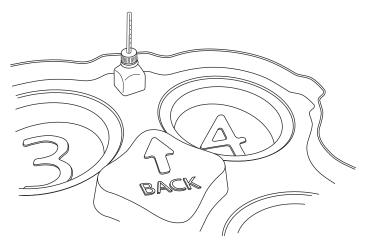
Figure 5-5 Temperature verification with the bottle locating base
