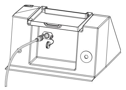
Figure 2-11 External device connection at rear of sampler
