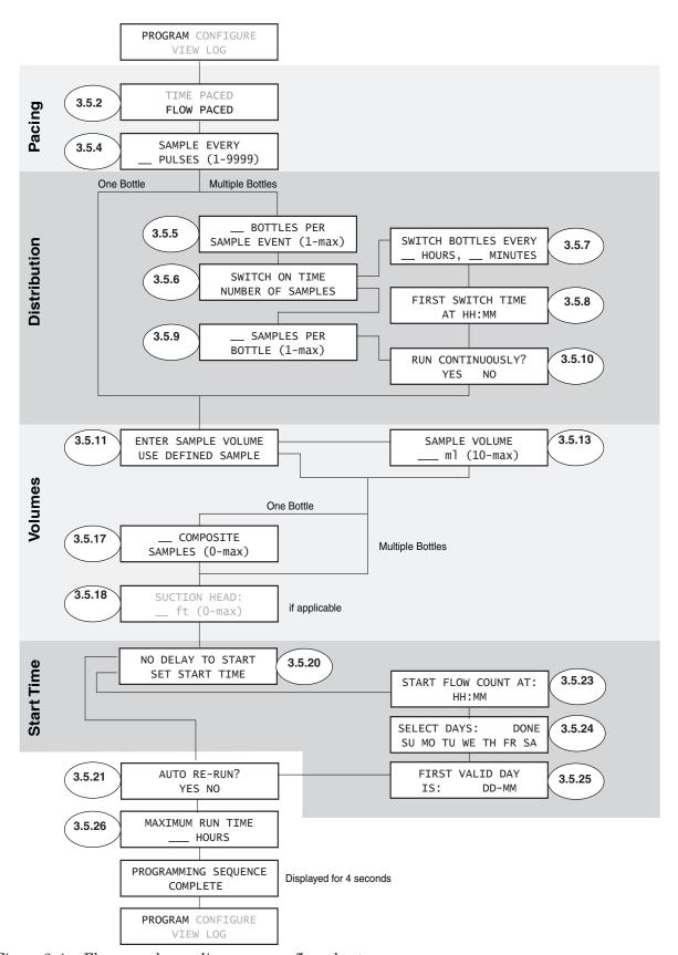
Figure 3-4 Flow paced sampling program flow chart
