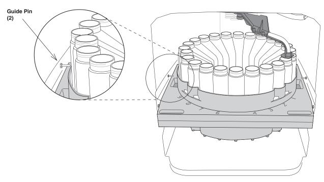
Figure 4-3 Sliding the 24-bottle rack out
