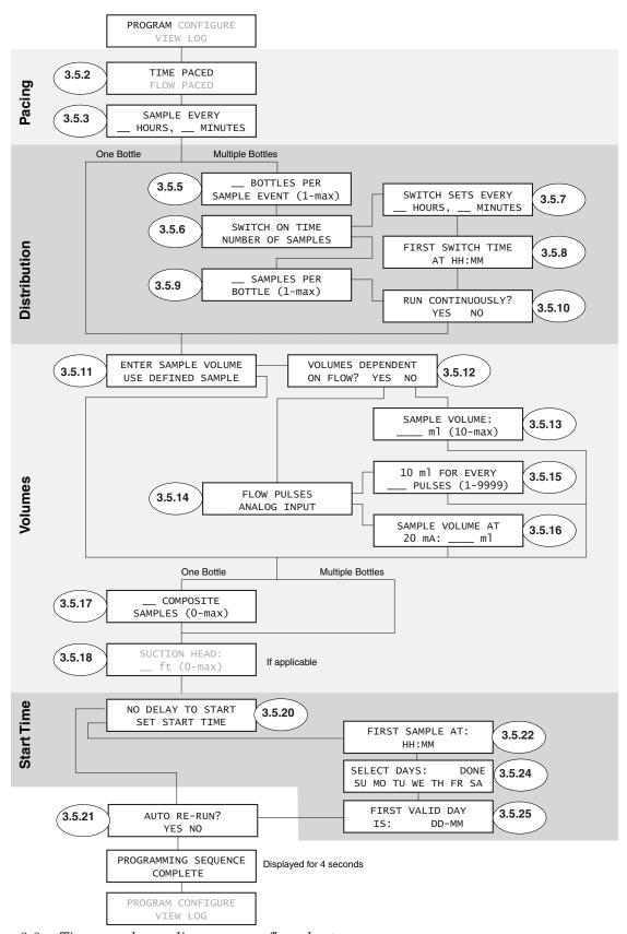
Figure 3-3 Time paced sampling program flow chart
