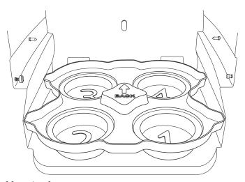
Figure 2-5 Installing the standard locating base
