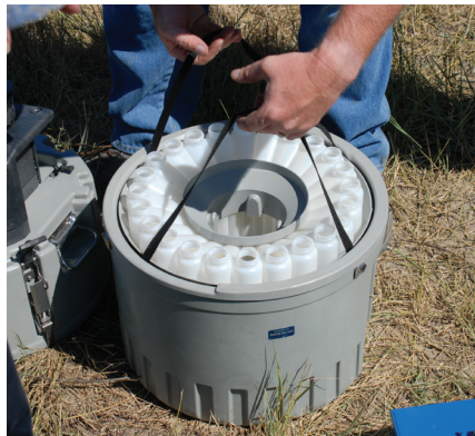
The 6712C Compact Portable Sampler features Teledyne ISCO's exclusive bottle carrier to make bottle changing and transportation a snap.
