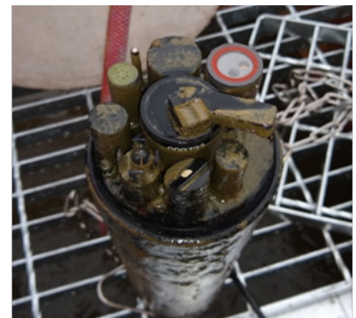
Above: A Proteus withdrawn from a PST tank showing the success of the wiper in maintaining a clear optical window for the TLF sensor!
