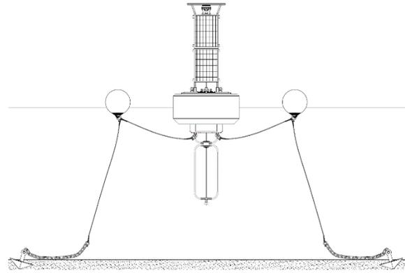
Used when monitoring sensors are deployed in the water column directly below the buoy
