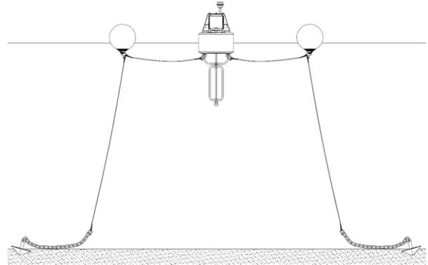
Used when monitoring sensors are deployed in the water column directly below the buoy
