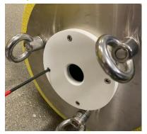
Carefully insert the sensor into the steel piping within the buoy.
