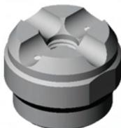
Hold the sensor firmly with the electrode tip facing upwards. Remove the existing salt bridge by using a 15/16 wrench (24mm) and turning it counterclockwise. Dispose of the salt bridge using an approved method.
