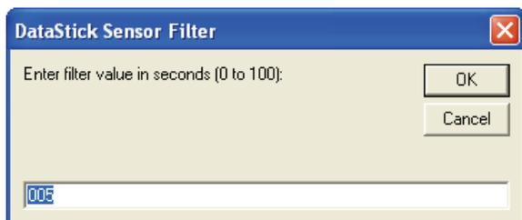
If the sensor filter is set to 5 seconds, it will take 5 seconds to reach 90% of the final value when the reading changes. Measurements are averaged to reduce periodic variations.
