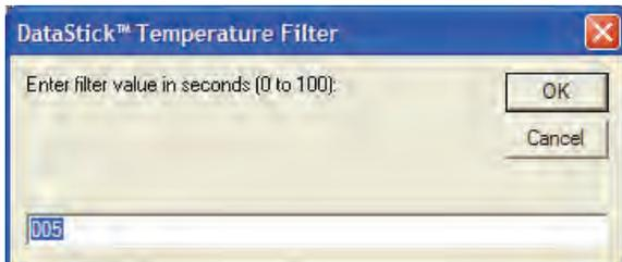
If the temperature filter is set to 5 seconds, it will take 5 seconds to reach 90% of the final value when the reading changes. Measurements are averaged to reduce periodic variations.
