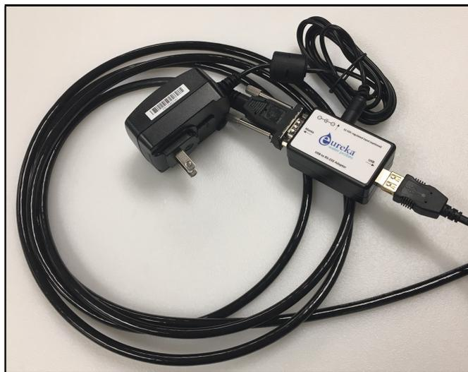
**Note: Do not connect your USB Adapter to any power source greater than 15 VDC unless that power source is protected by a ground-fault interrupter (GFI). GFI's are inexpensive and a necessary safety precaution.**
