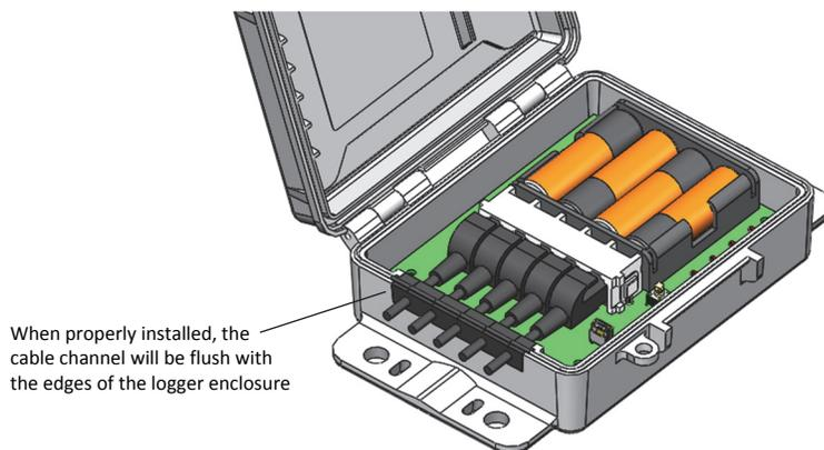
f. If you will be using less than five smart sensors, use the rubber plugs to fill any empty holes in the cable channel. Lightly coat the rubber plugs with a small amount of grease. Insert the thin part of the plug into the hole. While pulling the thin end of the plug from the inside of the case, push the other end of the plug from the outside until the thick part of the plug fills the hole.
