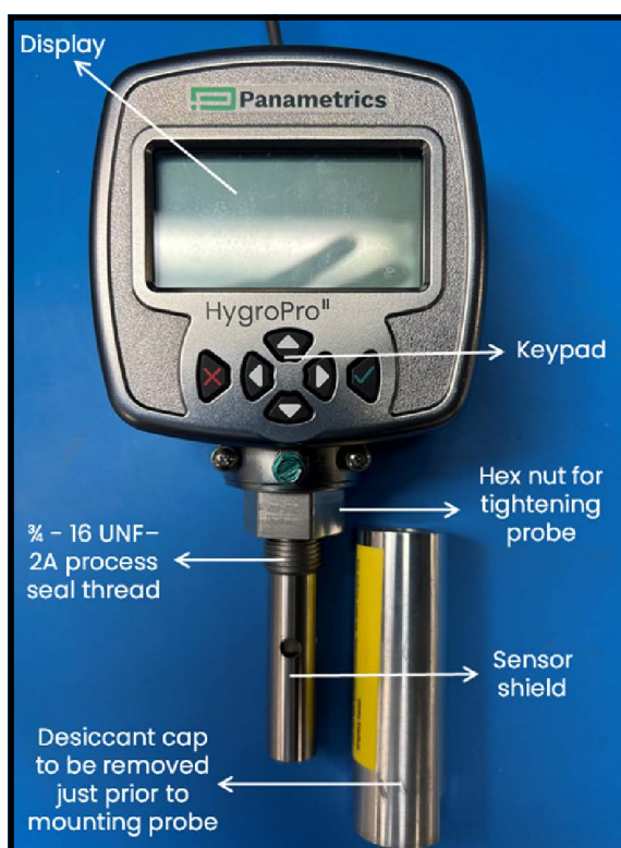
Figure 3: Key HygroPro II parts relevant to installation
