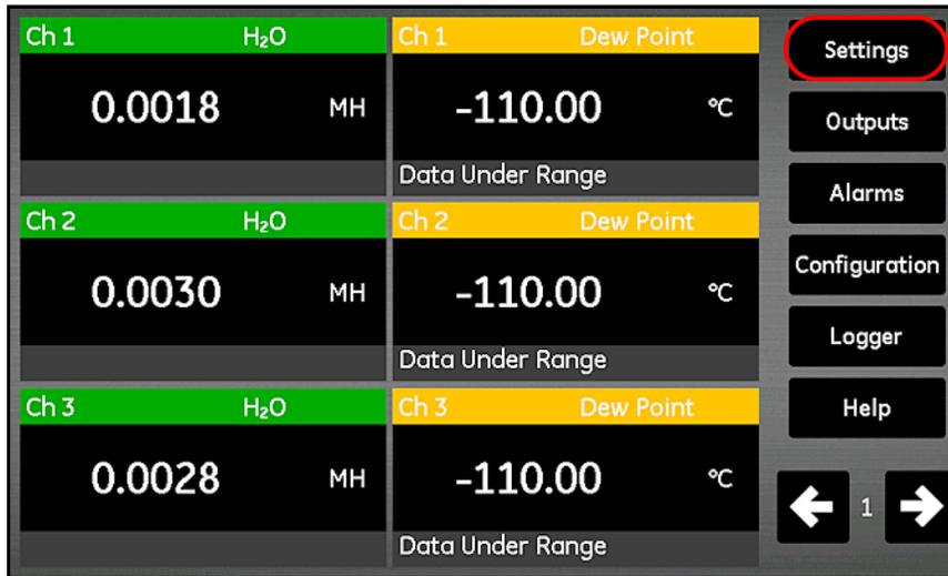
Figure 86: Settings Button on the Main Screen
