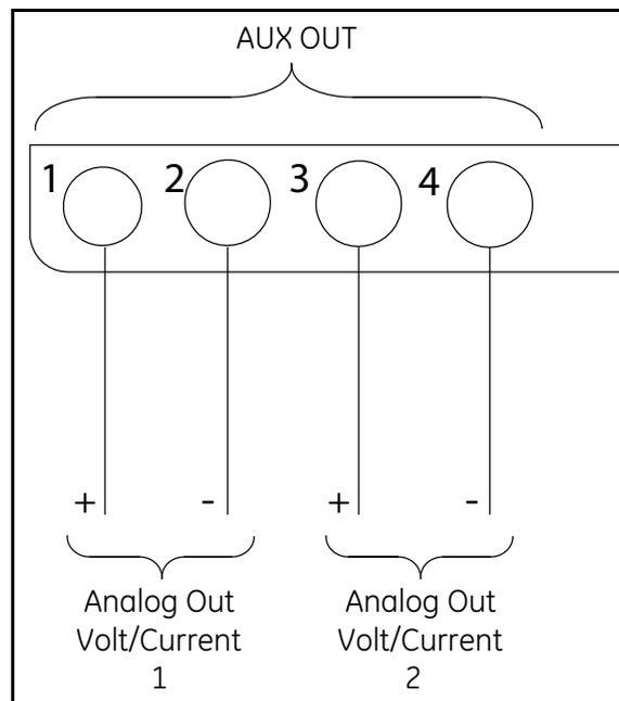
**Figure 25: Output Wiring**
