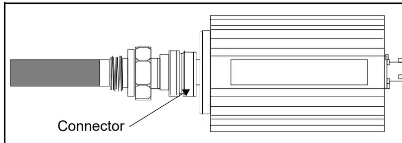
Figure 14: Moisture Image Series Probe (MISP) Assembly
