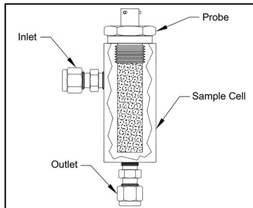
**Figure 4:** Typical Moisture Probe in Sample Cell
