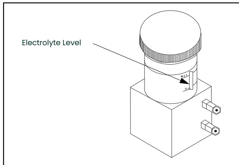
**Figure 7: Delta F Oxygen Cell Electrolyte Level**
