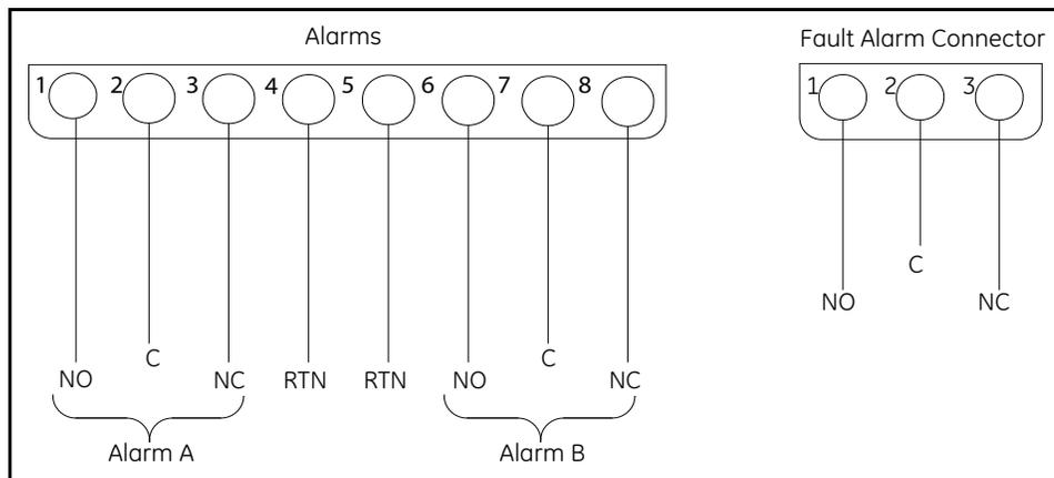
**Figure 26: Alarm Wiring**
