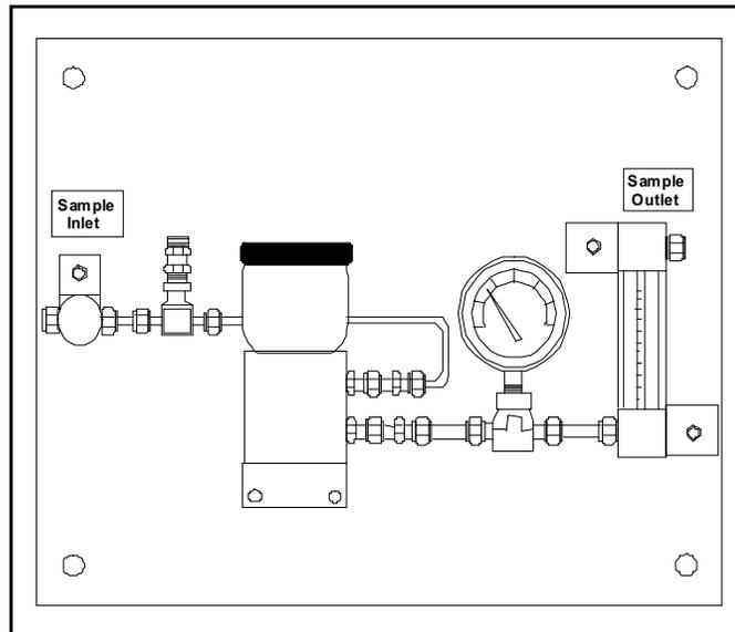
**Figure 2: A Typical Oxygen Cell Sample System**
