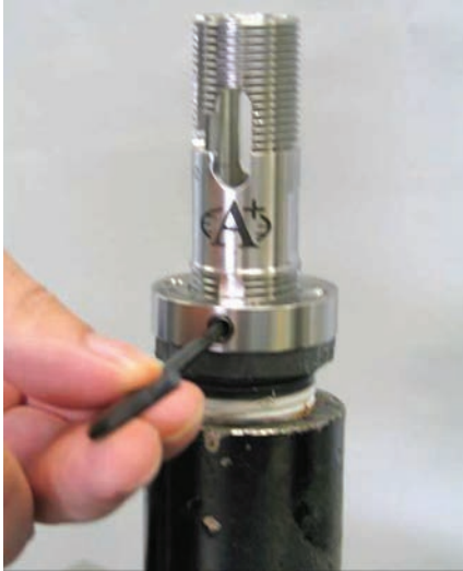
Figure 14: Aligning and tightening the Allen screw
