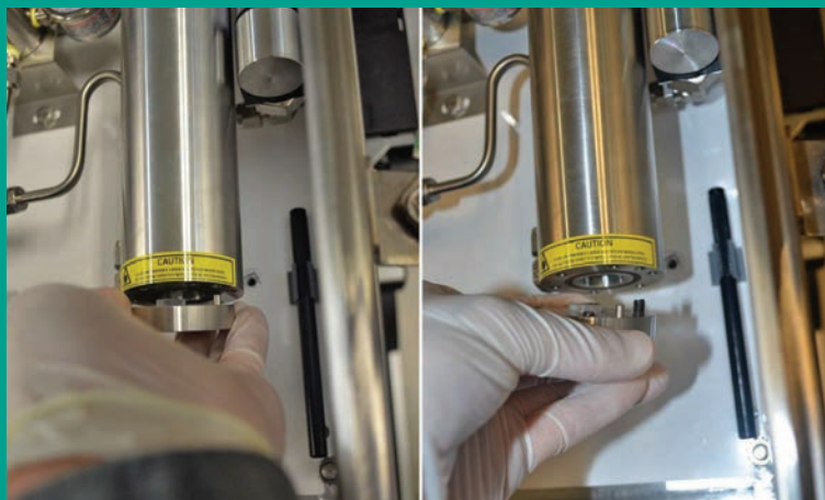
Figure 86: Reinstalling the mirror end cap assembly
