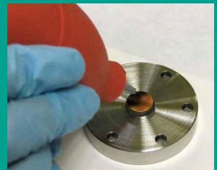
Figure 82: Blowing air onto the mirror
