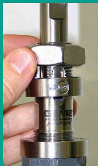
Figure 21: Loosening the insertion nut
