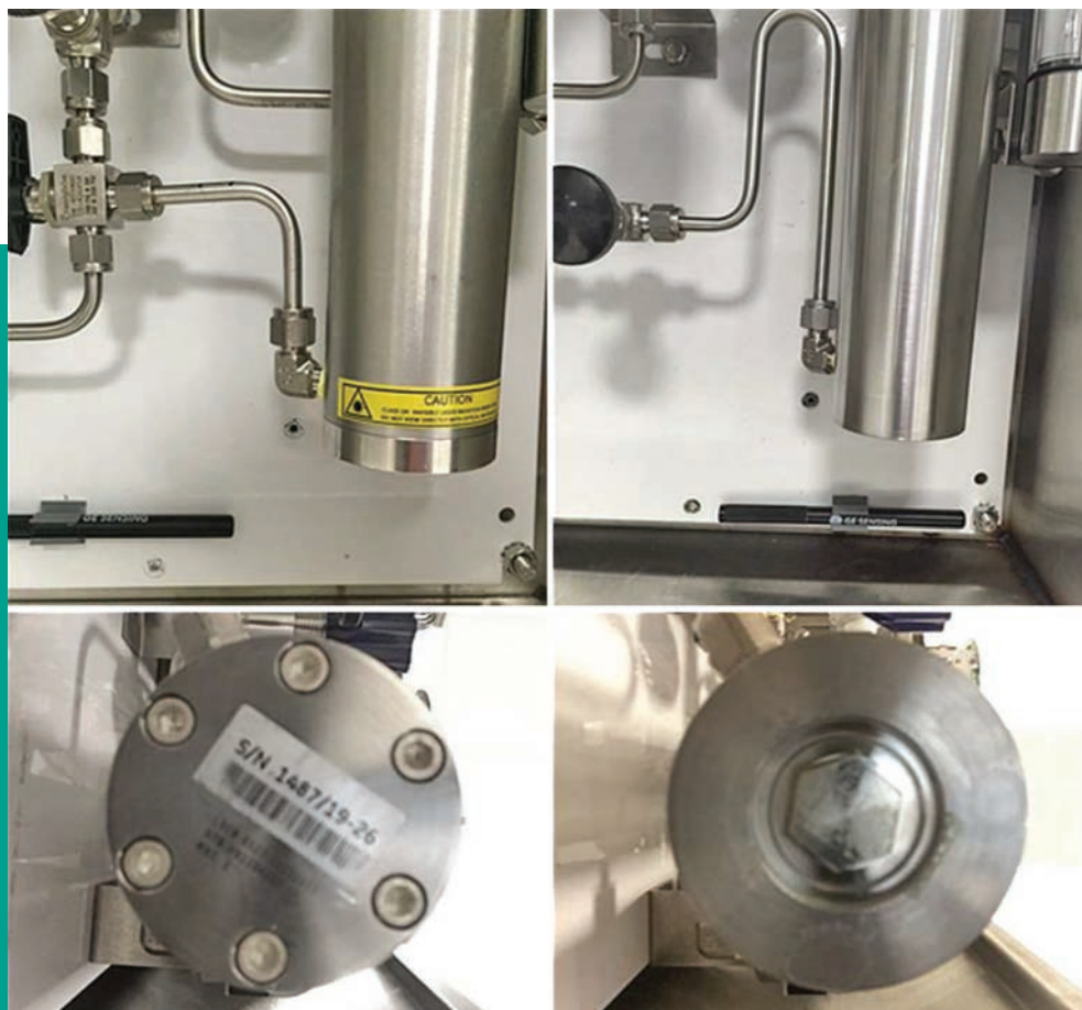
Figure 78: Style 1 (left) and style 2 (right) optical absorption cell/mirror assemblies
