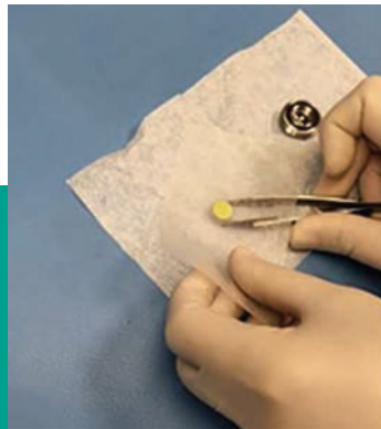
Figure 90: Cleaning a contaminated mirror
