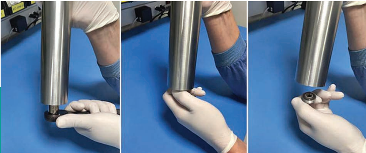
Figure 87: Removing mirror end cap assembly from the absorption cell
