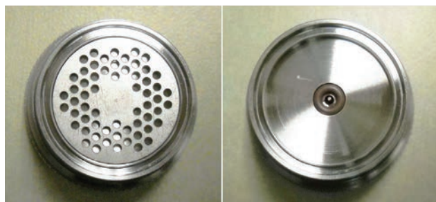
Figure 96: Remove the white filter element and the backing plate
