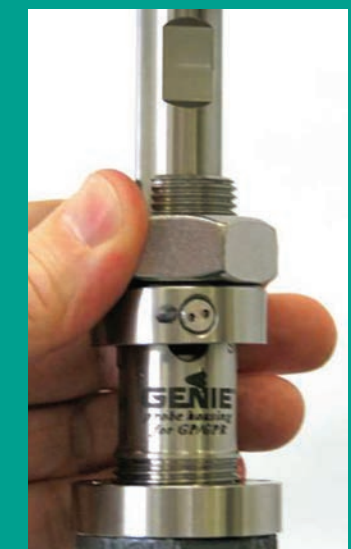
Figure 22: Tightening the insertion nut
