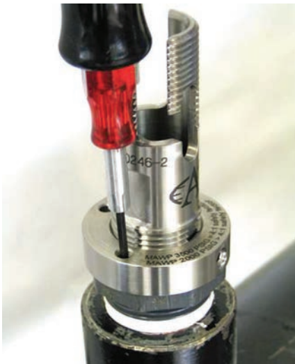
Figure 15: Tightening the Allen screws
