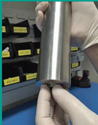
Figure 92: Replacing mirror end cap assembly into the absorption cell
