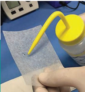
Figure 89: Applying acetone to lens tissue
