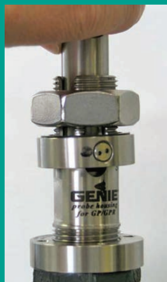
Figure 20: Rotating the probe
