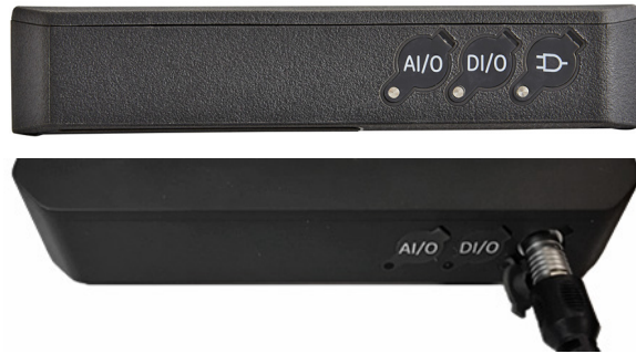
Figure 44: Transmitter power connection (right side)
