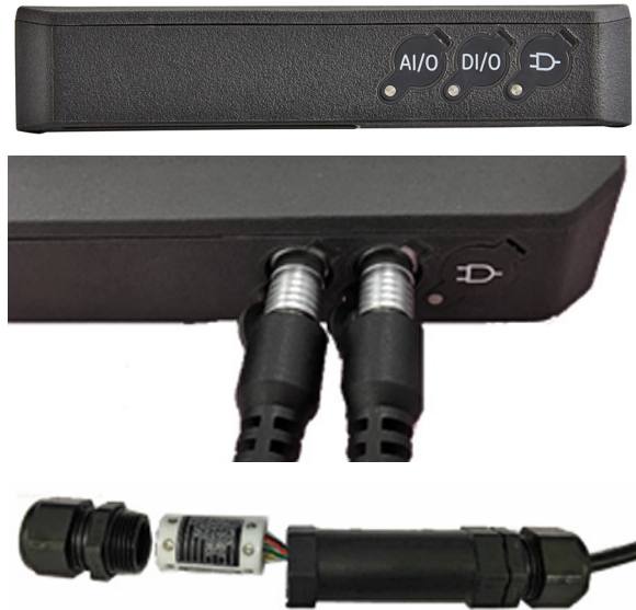
Figure 46: Transmitter I/O connections (right side)
