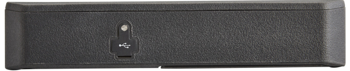
Figure 48: Transmitter USB connector (left side)
