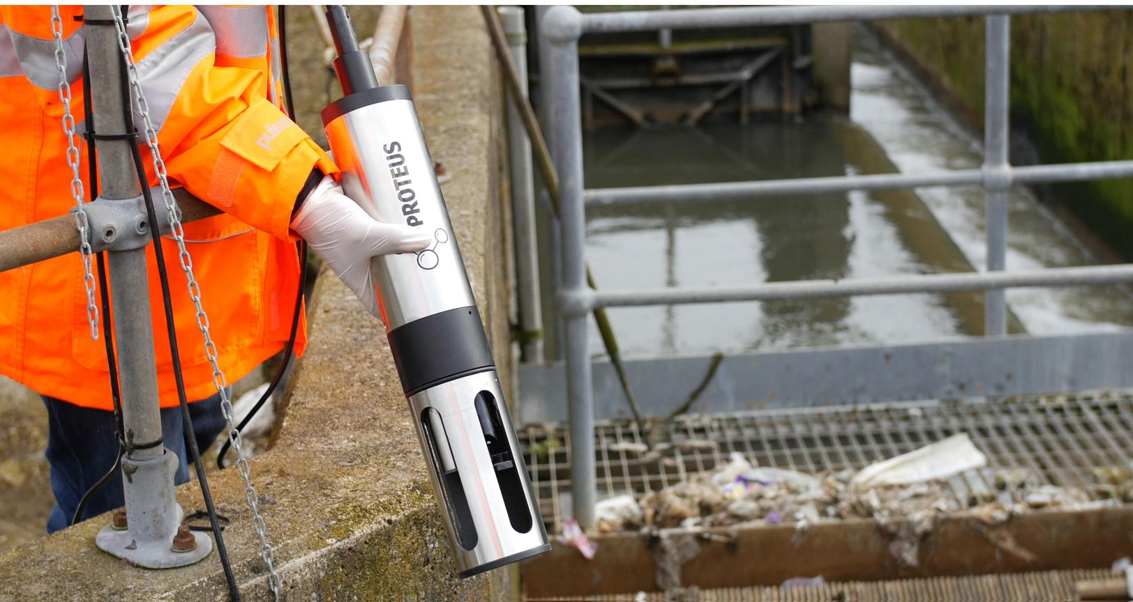
Self cleaning: As it is essential that optical sensors have a cleaning mechanism, the Proteus is also supplied with an integral wiper which cleans all of the Proteus' sensors before every measurement cycle.
